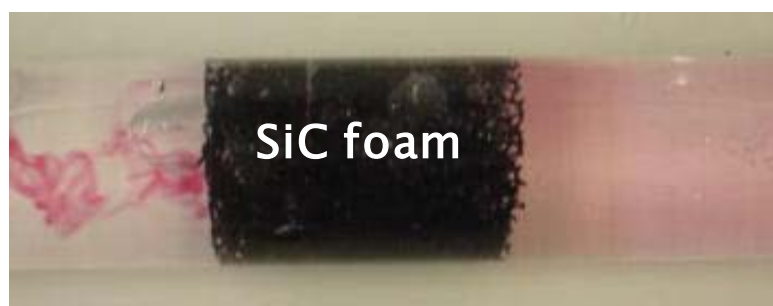
Figure 1-10. (A) Optical photo of the medium to high specific surface area (from 10 to 100 \text{ m}^2 \cdot \text{g}^{-1} ) porous silicon carbide support with different macroscopic shapes ranged from 10^{-6} \text{ m} to 10^{-1} \text{ m} . (B) Flow mixing through a SiC foam which acting as a static mixer. Courtesy by SICAT SARL. [136]
