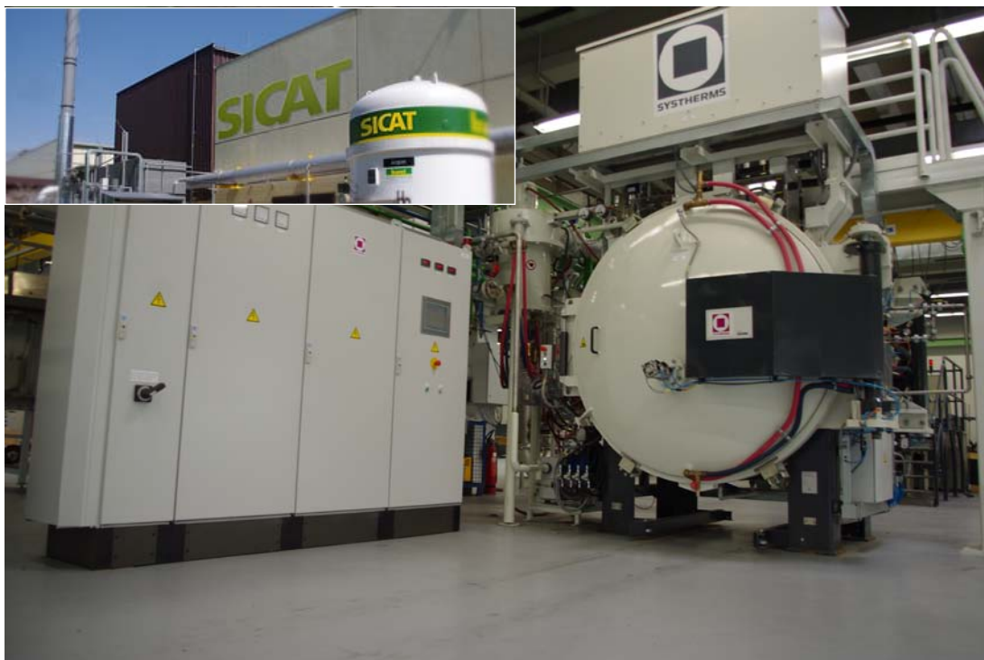
Figure 1-11. Pilot plant used for the industrial production of \beta -SiC according to the gas-solid reaction between SiO and solid carbon with a production capacity of 50 tons/year. Courtesy by SICAT SARL ( www.sicatcatalyst.com ).
