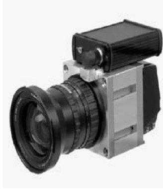
FIGURE 2.3: Rollei AIC digital aerial camera [Lemmens, 2008].
