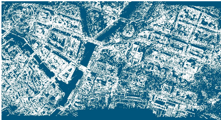
FIGURE 5.16: 3D point clouds produced from Rollei image (746,475 points).
