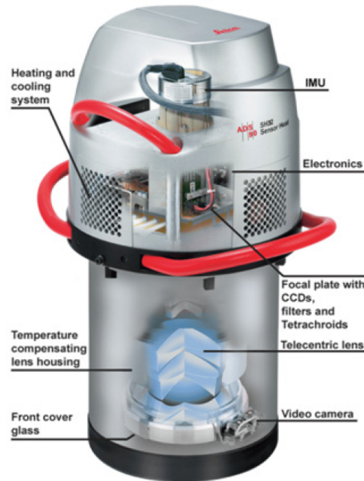
FIGURE 2.9: Airborne linear cameras: ADS80 [Wagner, 2011a].
