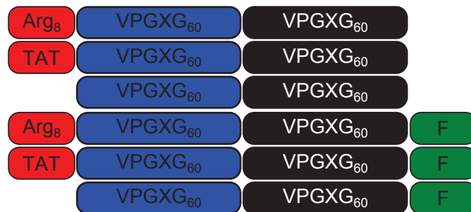
Figure 3.11: Peptide sequence of Arg 8 and TAT-functionalized ELP BC with and without a fluorescent label. Non-functionalized ELP BC was used to compare interactions of ELP BC without a CPP residue.
