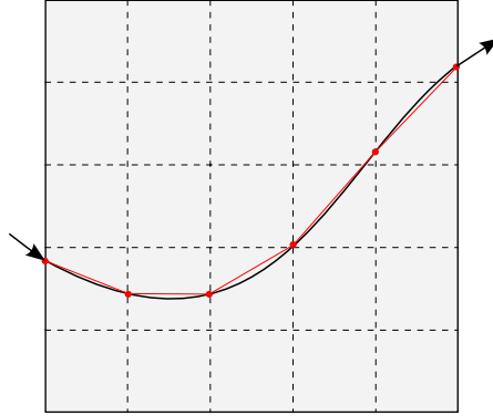
Figure 3.14: Illustration of a raytracing on a curved trajectory.
