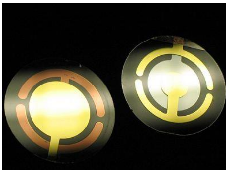
Figure 2.14: Schematic representation of a QCM-D quartz crystal sandwiched by two gold layers. The larger gold electrode on the left is the one in contact with the solution. The gold electrode displayed on the right is in contact with the electronic card controlling the EC-QCM-D.
