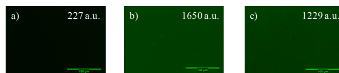
Figure 2: Fluorescence microscopy images taken from modified silicone surface after contact with (a) GFP wt, (b) N_3 -GFP (39) and (c) N_3 -GFP- N_3 (39, 182). The values written in white is the quantification of the fluorescence evaluated in arbitrary unity (a.u.) by using ImageJ software but comparable one to each other.
