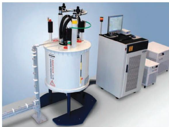
Figure 2.16: Photograph of the Bruker Biospin 263 GHz gyrotron showing from left to right: microwave transmission line, gyrotron magnet with tube installed, gyrotron control system console, and two chiller units. Taken from Rosay et al 2010
