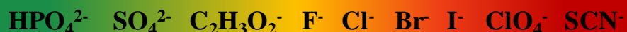
Figure 1.16: Hofmeister series: ranking of anions by their hydration degree. The hydration degree is decreasing from the left to the right of the scheme.
