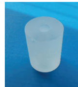
FIGURE 3.5: The cylinder is introduced in a 50 ml tube held cover-slips in a vertical position.
