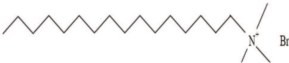
Figure 25 : structure d'hexadecyl trimethylammonium bromide CH 3 (CH 2 ) 15 N + (CH 3 ) 3 Br -
