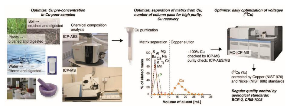
**Figure II-1:** Schematic of the different steps of the methodology applied and adapted in this thesis to measure Cu isotope ratios in soil, sediment, vegetal, and water samples.
