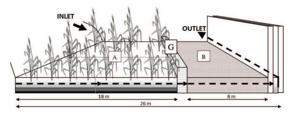
**Figure IV-2:** Scheme of the constructed stormwater wetland (Rouffach, France, year of construction 2002). The wetland is composed of a vegetated forebay (A) and the gravel filter (B), separated by a gabion barrier (G), a box filled with rocks whose role is to enhance the dispersion of water ahead of the gravel filter.
