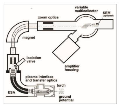
**Figure II-8:** The schematic image of a double focusing multicollector ICP-MS (ESA: Electric sector analyzer (Figure from Goldstein and Stirling, 2003).<sup>36</sup>
