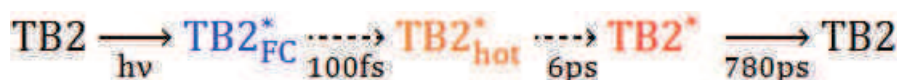
Figure 5.13.: Reaction scheme describing TB2 photochemistry in solution in chloroform upon 600nm excitation. Dotted arrows indicates vibrational relaxations, plain arrows electronic transitions.
