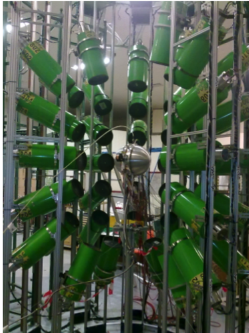
Figure 2.1: Experimental set-up: 60 DEMON cells are arranged on the surface of a sphere intercepting neutrons. The CODIS fission chamber is mounted at the centre of the sphere.
