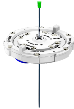
Figure B.1 – Second version of the needle MRE driver, based on a ring-shaped piezoelectric actuator.
