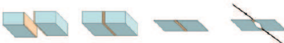
Figure 3-9 (b). Preparation of a sample for TEM cross section observation , with the ion milling a the last step.
