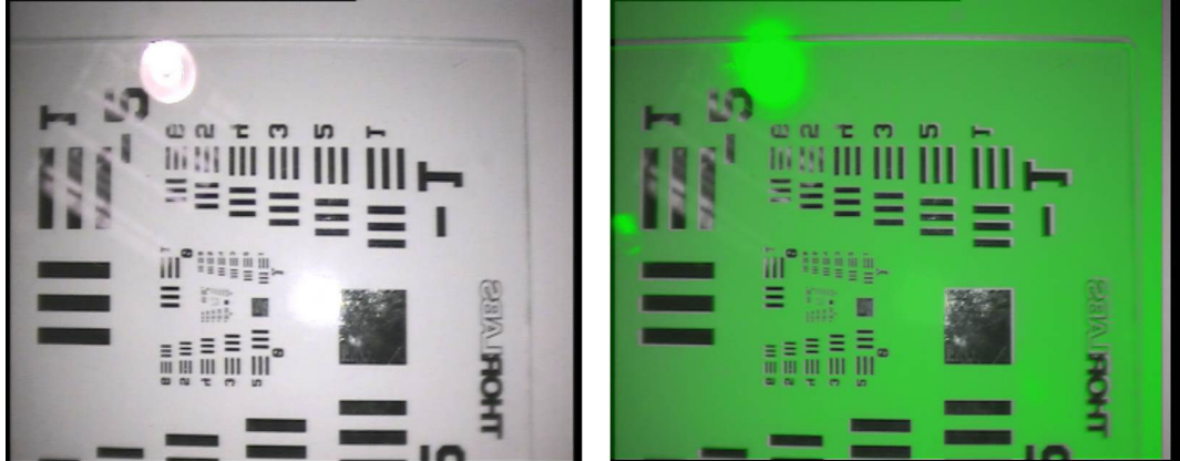
Figure 3.23: Views of a USAF1951 standard resolution target. On the left, the color channel only. On the right, color and fluorescence channel (green) using an additional NIR light
