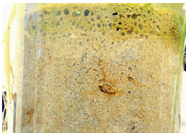
Figure III-11. Reddish-brown ferric iron oxide precipitates along Phragmites australis root periphery in a lab-scale wetland.
