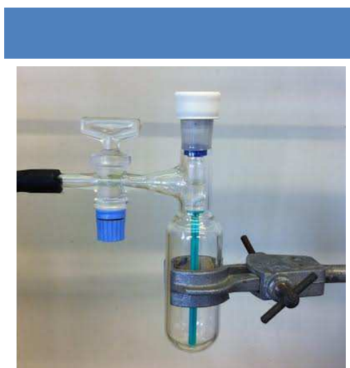
Figure 12 | Picture of the setup: the HPLC vial containing the stirring bar and the exchange reaction solution is inserted in a Schlenk tube.
