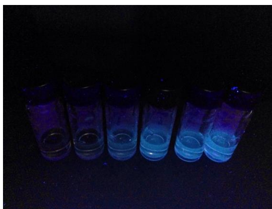
Figure 2.2. Different fractions of Si NPs separated by DGU under UV irradiation (the blue emission comes from the fractions containing the nanoparticles)
