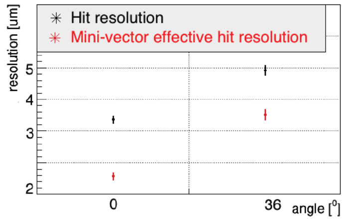
Figure 5.24: Resolution measured along the v direction, for tilts = 0^\circ and 36^\circ (sensor 2).
