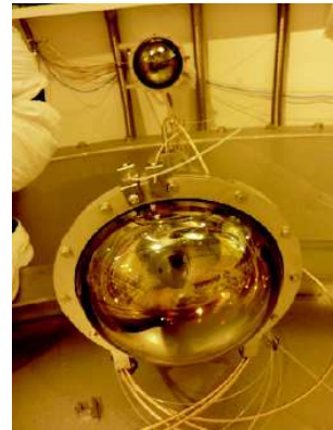
(c) A PMT with two fibres attached.
