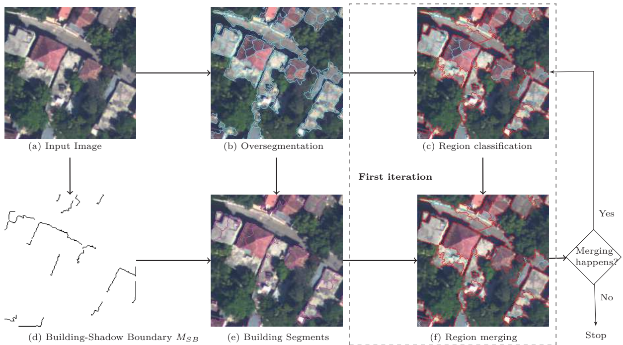
Figure 5.7: An example of the first iteration of the region growing image segmentation method: (a) input image, (b) SLIC oversegmentation (regions are separated by cyan lines) of the image in which shadow regions M_S and vegetation regions M_v are masked out, (c) MRF-based classification (clusters are separated by red lines), (d) Building-Shadow boundary mask M_{SB} (see Section 5.4), (e) detected building segments (boundaries are delineated by violet lines), (f) after merging (some cyan lines are disappeared).
