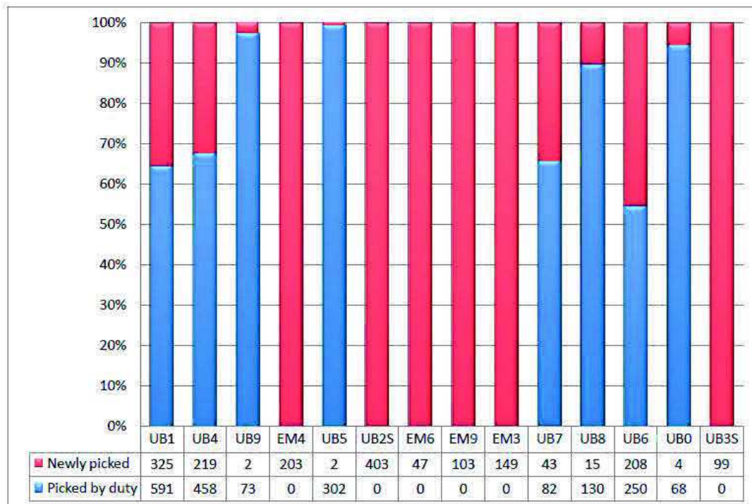
Figure 3.5. The phase picking percentage of events between 2011.08 and 2013.01 per station. All these stations are mobile stations. Blue colour represents phase picking by the duty at NDC and red colour represents my newly picked phases. The order of the stations, from left to right, is by increasing distance from the central point of the study area (47.9N, 106.6E)
