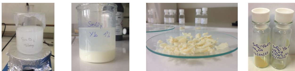
Figure 3.1 Different steps of synthesis of the RE doped SnO 2 powders by the co-precipitation method
