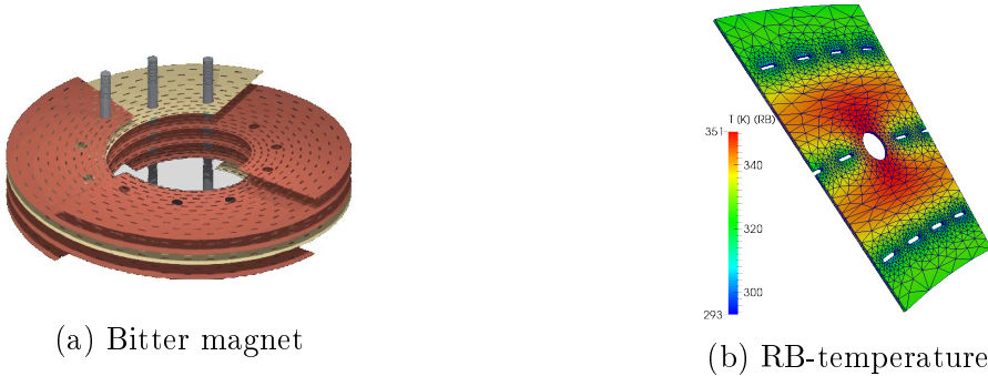
Figure 4.1 – RB approximation on a sector of a Bitter magnet
