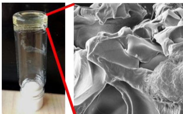
Figure 2.4 Hydrogel containing \gamma -aminobutyric acid as co-monomer; inverted vial test and SEM morphological characterizations.
