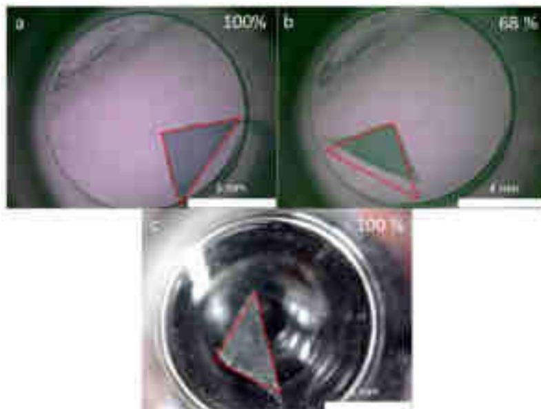
Figure 106 | Snapshots from a video of the contraction of a piece of Gel 25 under irradiation at 312 and 365 nm, with their relative volume, a) before experiment, b) after contraction, c) after extension when exposed to visible light. The red triangle represents the size of the original piece of gel, and has the same dimension on every picture.
