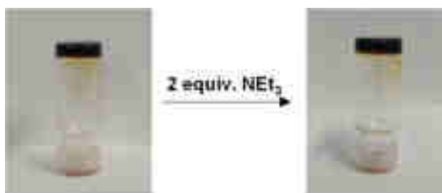
Figure A 4 | Behavior of 18 wt. % gel of 46^{\text{Ext-G}} in toluene upon addition of two equivalents of triethylamine.
