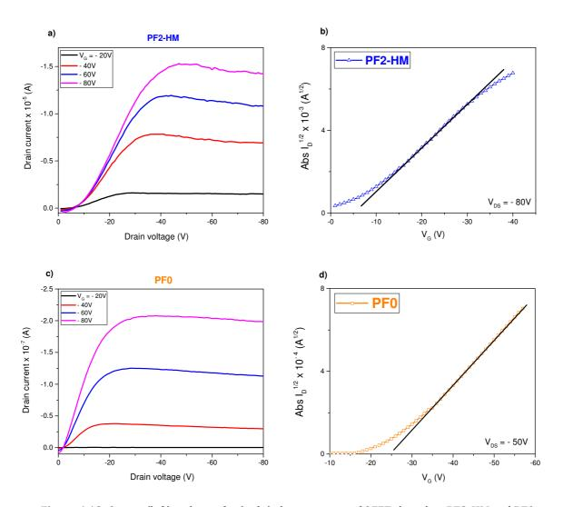
**Figure 6.18:** Output (left) and transfer (right) characteristics of OFETs based on **PF2-HM** and **PF0** copolymers. Black solid lines represent the slopes used to estimate hole mobility values
