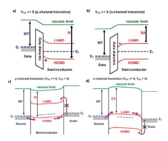
**Figure 3.9:** Energy-level diagrams a) and b) after applying  $V_G$  via organic layer/dielectric interface, showing the accumulation of holes and electrons, respectively; c) and d) along the channel after applying the  $V_{DS}$  showing the drift of holes and electrons, respectively. Reproduced from Ref [141].
