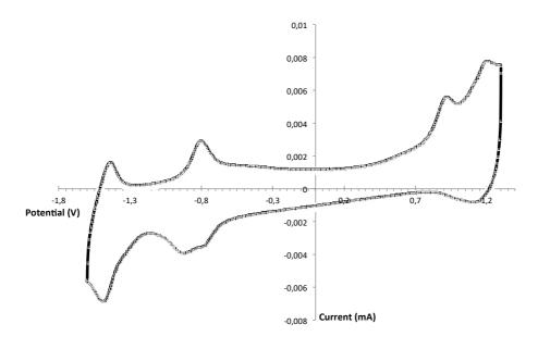
Fig. S2. Cyclic voltammogram of PPPyT² in solid state
