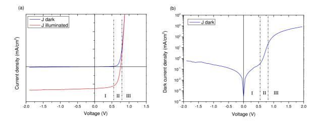
**Figure 2.5**: (a) An exemplary current density-voltage curves under dark (blue) and illuminated (red) conditions; (b) the dark current density of a solar cell plotted versus voltage using absolute values in a semi-logarithmic scale. Three different regions I, II and III can be distinguished where the behavior is dominated by  $R_{sh}$  (I)  $R_s$  (III) or where a perfect diode can be assumed (II), respectively.
