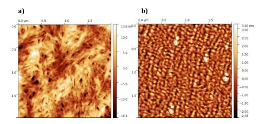
**Figure 6.23:** AFM images of a) **PF2-MM**:PC[71]BM and b) **PF0**:PC[71]BM thin films. D:A ratio in both cases was 1:1.5
