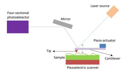
Figure 3.11: A simplified scheme of an AFM assembly
