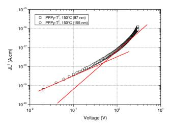
Fig. S9. SCLC characteristics of pure, annealed PPPyT $^2$  films (open symbols) with two different thicknesses. Solid lines represent ohmic part (J  $\bigcirc$  V) and space-charge limited part (J  $\bigcirc$  V $^2$ ) dependence
