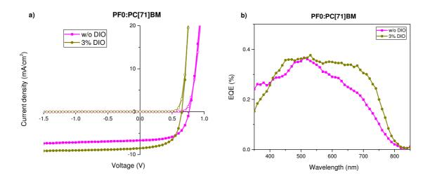
**Figure 6.16:** a) (J-V) characteristics in the dark (open symbols) and under standard AM1.5G (100 mW/cm<sup>2</sup>) illumination (closed symbols) and b) EQE curves of **PF0:PC[71]BM** solar cells processed with or without additives (D:A ratio is 1:1.5)
