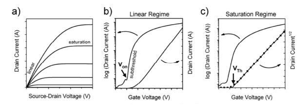
**Figure 3.10:** Current-voltage characteristics for OFETs: a) Output characteristics with the linear and saturation regimes; Transfer characteristics in b) linear regime with onset voltage ( $V_{on}$ ) and c) saturation regime indicating threshold voltage ( $V_{Th}$ ). Reproduced from Ref. [142].
