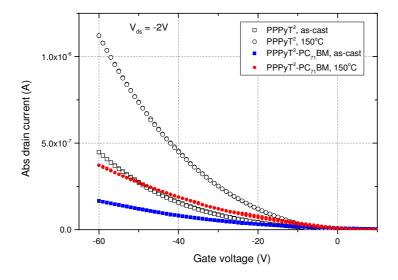
Fig. S6. Transfer characteristics of pure  $PPPyT^2$  film and  $PPPyT^2:PC_{71}BM$  blend as-cast and annealed at  $150^{\circ}C$  for 15 mins. Drain-source voltage  $V_{ds}$  is set to -2V
