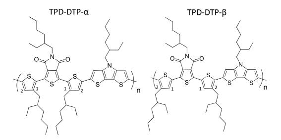
**Figure 4.1**: Chemical structures of TPD-DTP- $\alpha$  (left) and TPD-DTP- $\beta$  (right) polymers. Positions 1 and 2 on the thiophene correspond to the  $\alpha$  and  $\beta$  polymers, respectively.
