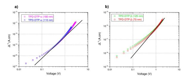
Figure 4.5: Current-voltage characteristics of hole-only SCL diodes based on a) TPD-DTP- $\alpha$  and b) TPD-DTP- $\beta$  for 2 different polymer layer thicknesses
