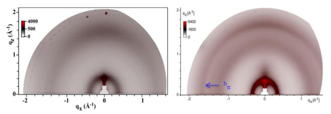
Figure 4.7: GIWAXS patterns of as-deposited TPD-DTP- $\alpha$  (left) and TPD-DTP- $\beta$  (right) pristine polymer films.
