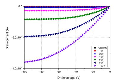
Fig. S3. Output characteristics of pure PPPyT<sup>2</sup> film annealed at 150°C for 15 min.
