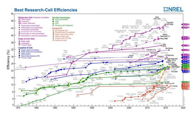
Fig. 1.1: Evolution of power conversion efficiencies of different types of solar cells versus time. Reproduced from reference [a].
