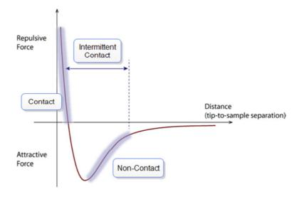
Figure 3.12: Tip-sample interaction as a function of spacing
