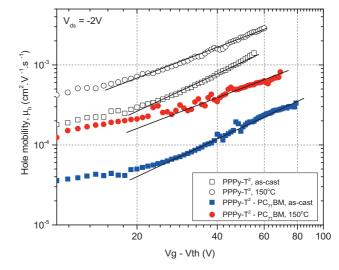
**Fig. 3.** Hole mobility  $(\mu_h)$  as a function of  $V_g - V_{th}$  for pure **PPPyT**<sup>2</sup> films (open symbols) and for **PPPyT**<sup>2</sup>–**PC**<sub>71</sub>**BM** blends (closed symbols) before (squares) and after annealing (circles).  $V_{th}$  for as-cast and annealed polymer films are +4 and 0 V, for blends are +7 and +17 V, respectively. Solid lines represent slopes to each of the curves
