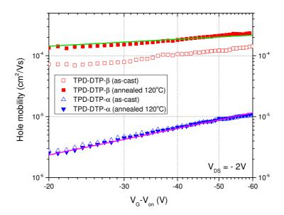
**Figure 4.4**: Evolution of  $\mu_{n,lin}^{FET}$  vs effective gate voltage for **TPD-DTP-β** (red) and **TPD-DTP-α** (blue) as-cast (open symbols) and annealed for 30 min at 120°C (closed symbols) devices. Solid lines stand as eye guides for the mobility dependence on the gate voltage
