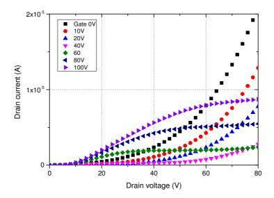
Fig. S5. Output characteristics of  $PPPyT^2:PC_{71}BM$  blend annealed at  $150^{\circ}C$  for 15 min at positive drain and gate voltages.
