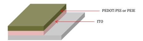
Figure 3.2: Schematic view of interfacial layers coated on ITO after cleaning from one side
