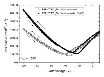
Fig. S7. Current-voltage characteristics of PPPyT<sup>2</sup>:PC<sub>71</sub>BM blends wt% ratio: 1/1 before and after annealing at negative gate voltages (for hole mobility in blends). Upper arrows show forward directions.
