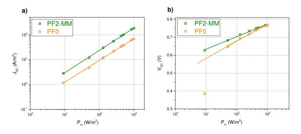
**Figure 6.25:** a)  $J_{SC}$  plots as a function of illuminated light power ( $P_{in}$ ) in log-log scale for both materials. Solid lines represent fits using power-law dependence for  $J_{SC}$  and  $P_{in}$  with a similar power of  $\approx 0.9$  for both; b)  $V_{OC}$  as a function of  $P_{in}$  for both copolymers. Solid lines are fits using single logarithmic laws described by the Eq. 6.1.
