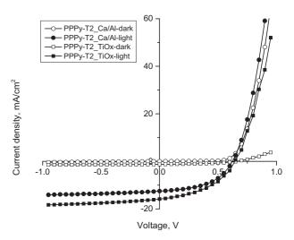
**Fig. 5.** Current–voltage curves of best photovoltaic devices under illumination (1,5AM) and dark conditions.
