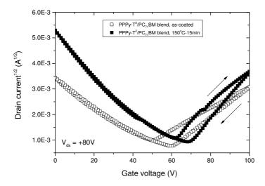
Fig. S8. Current-voltage characteristics of PPPy- $T^2$ :PC<sub>71</sub>BM blends at positive gate voltages (for electron mobility). Upper arrow indicates the forward direction, and the below one backward direction
