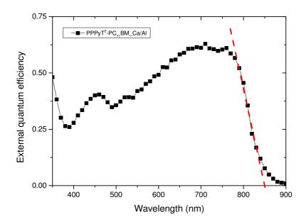
Fig. S11. EQE spectrum of best PPPyT<sup>2</sup>:PC<sub>71</sub>BM device with Ca/Al cathode. Dashed red line represents the extrapolation of the onset to estimate the band gap
