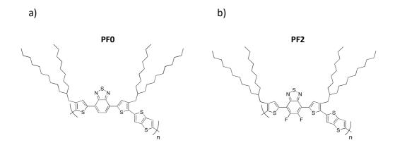
Figure 6.13: Chemical structures of a) non-fluorinated PFO and b) fluorinated PF2
