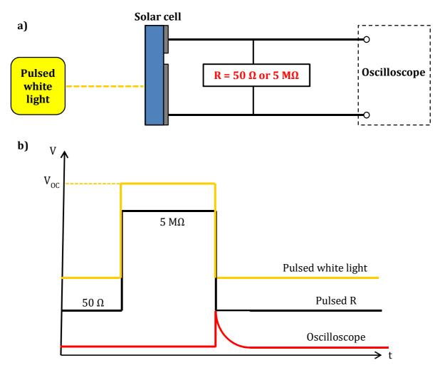
**Figure 3.6:** Scheme of a) CE setup at the ICube; b) measured current drop (in red) after switching to short circuit condition
