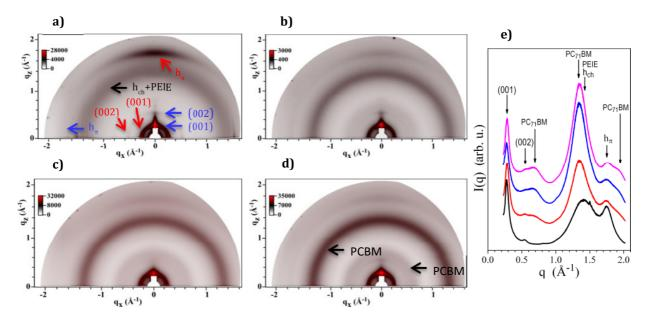
**Figure 6.22:** GIWAXS patterns of a) pure **PF0** copolymer; b) **PF0**:PC[71]BM at 1:1 ratio; c) 1:1.5 ratio; and d) 1:2 ratio. e) Radial profiles of GIWAXS patterns of pure polymer film (black), polymer:fullerene blend film ratio of 1:1 (red), 1:1.5 (blue) and 1:2 (magenta)
