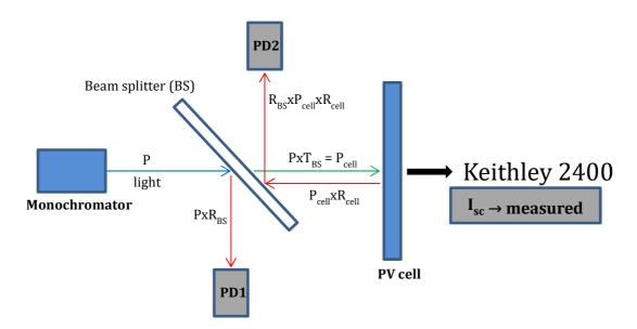
**Figure 3.4:** Schematic view of EQE/IQE measurement setup at ICube. P – power of incident light; PD1 – photodiode 1; PD2 – photodiode 2;  $T_{BS}$  and  $R_{BS}$  – transmittance and reflectance of the beam splitter, respectively;  $P_{cell}$  and  $R_{cell}$  – light power incident to PV cell and reflectance of PV cell, respectively;  $I_{sc}$  – measured short circuit current.
