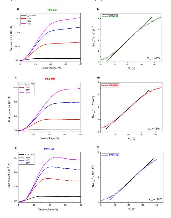
**Figure 6.6:** Output (left) and transfer (right) characteristics of **PF2** copolymers of different molecular weights. Black solid lines represent the slopes used to estimate hole mobility values
