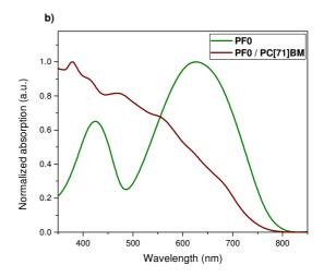
**Figure 6.15:** Absorption profiles of thin films based on a) **PF2-HM** and b) **PF0** copolymers in pure materials (green) and BHJ blends (brown) at a polymer:fullerene ratio of 1:1.5
