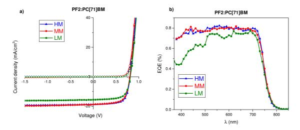
**Figure 6.4:** a) (J-V) characteristics in the dark (open symbols) and under AM1.5G ( $100 \text{ mW/cm}^2$ ) conditions (closed symbols) and b) EQE curves of BHJ devices based on different molecular weight fluorinated polymers
