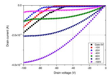
Fig. S4. Output characteristics of  $PPPyT^2$ :  $PC_{71}BM$  blend annealed at  $150^{\circ}C$  for 15 min at negative gate voltages.
