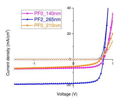
**Figure 6.17:** (J-V) characteristics in the dark (open symbols) and under standard AM1.5G ( $100 \text{ mW/cm}^2$ ) illumination (closed symbols) for the best BHJ devices for the fluorinated polymer and two active layer thicknesses for the non-fluorinated one.
