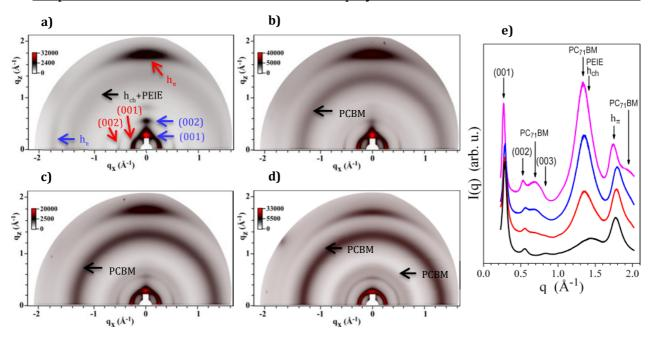
**Figure 6.12:** GIWAXS patterns of a) pure **PF2-HM** copolymer; b) **PF2-HM**:PC[71]BM at 1:1 ratio; c) 1:1.5 ratio; and d) 1:2 ratio. e) Radial profiles of GIWAXS patterns pure polymer film (black), polymer:fullerene blend film ratio of 1:1 (red), 1:1.5 (blue) and 1:2 (magenta)
