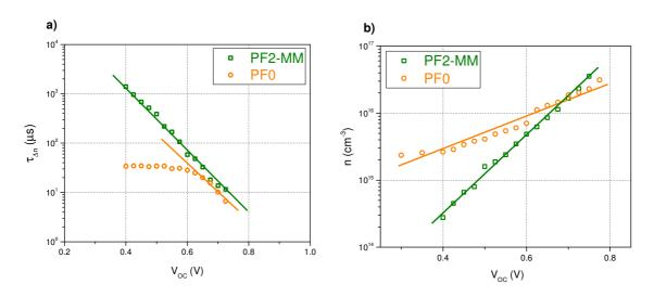
**Figure 6.26:** a) Dependences of charge-carrier recombination time in small perturbation regime  $(\tau_{\Delta n})$  versus  $V_{0C}$ . Best fits using Eq. 6.2 are shown in solid lines with fitting parameters in Table 6.9; b) Charge-carrier concentration n as a function of  $V_{0C}$ . Solid lines are the best fits using the Eq. 6.3 with fitting parameters listed in Table 6.9.
