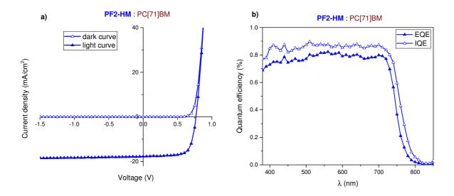
**Figure 6.5:** Best recorded a) (J-V) characteristics and b) quantum efficiency curves of solar cells based on **PF2-HM**:PC[71]BM blends
