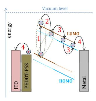
**Figure 2.2**: Schematic view of four crucial physical steps in organic solar cells: 1) light absorption and exciton generation; 2) exciton diffusion and dissociation at the donor/acceptor interface; 3) charge transport; 4) charge collection at the electrodes. The brown color refers to the electron-donor material and the blue color to the electron-acceptor material.
