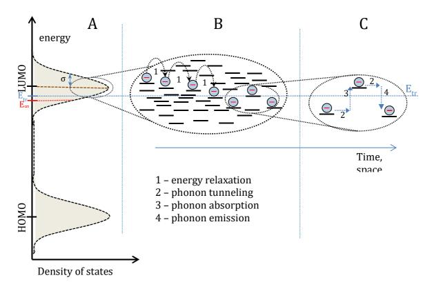
**Figure 2.3**: A) Distribution of density of states, inset: density of occupied states (DOOS) B) energy relaxation of an electron in excited state by hopping to energetically favorable sites; C) electron transport within the transport energy level ( $E_{tr}$ ).  $\sigma$  and  $T_0$  – width of Gaussian and Exponential DOS, respectively.
