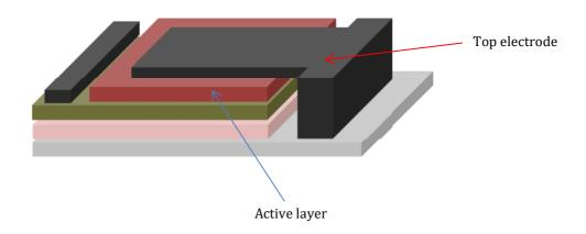
Figure 3.3: Schematic view of final photovoltaic device
