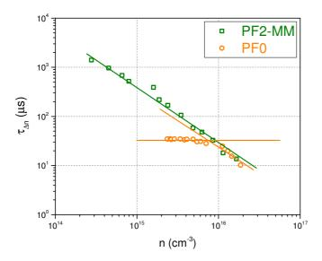
Figure 6.27: Dependence of charge-carrier recombination time in small perturbation regime  $(\tau_{\Delta n})$  versus the charge-carrier concentration n for both copolymers. Solid lines are the best fits to the experimental data points using Eq. 6.4
