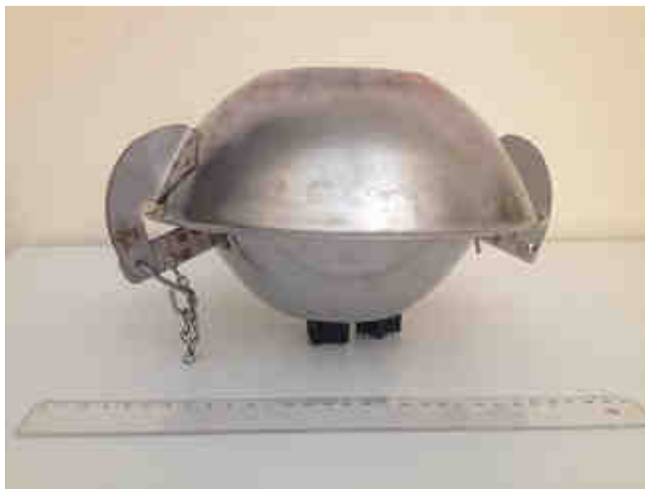
Figure 1-1 – Stainless steel 'flying saucer' protecting a PUF disk
