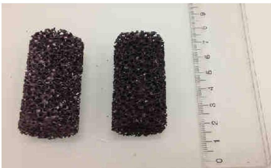
Figure 1-9 – SiC foam (left) and N-CNT SiC foam (right)
