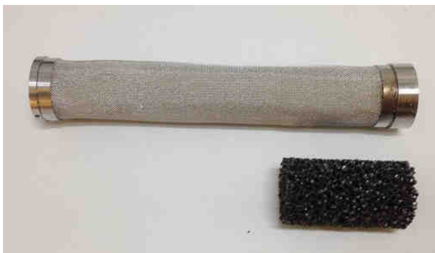
Figure 2-1 – Relative sizes of XAD®-2 resin tubes and SiC foams
