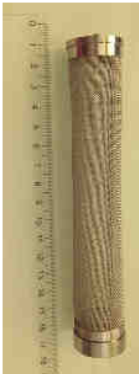
Figure 1-4 – Meshed cylinder to be filled with XAD®-2 resin
