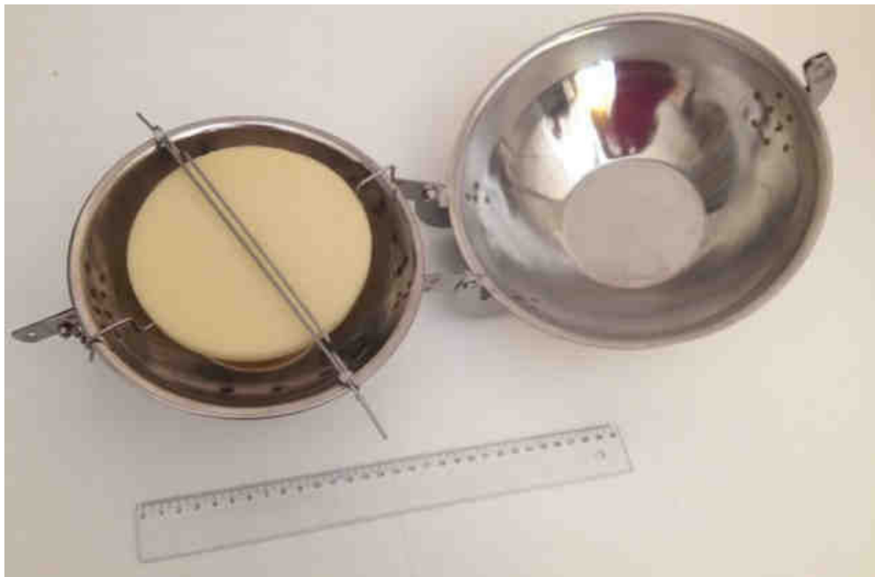
Figure 1-2 – Placement of a PUF disk inside its housing
