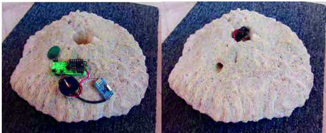
Figure 5.6 Arduino on the rocks. An actual seabed rock perforated to be loaded with an Arduino data logger.
