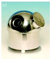
Figure 4.21: SR-PES endstation of the CASSIOPÉE beamline. Picture of (a) the SR-PES-dedicated endstation, (b) the sample inside the SR-PES measurement chamber (in the back visible input of the energy-analyzer), and (c) the Mott detector with one of the channelplates removed. Pictures taken from ref. 235 and 236.
