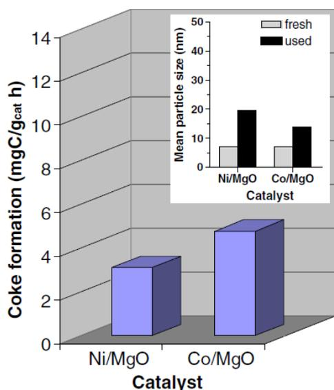
**Fig. 1.6** Coke formation (evaluated by Carlo-Erba elementary analyser) and mean particle size (evaluated by TEM) of Ni/MgO and Co/MgO catalysts after 20 h ESR. Based on Fig. 5 and 6 from F. Frusteri et al. studies [70].
