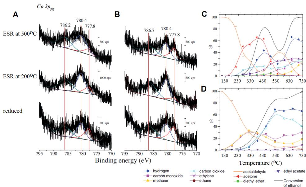
**Fig. 1.20** The peak fitting of Co 2p<sub>3/2</sub> spectra after reduction and after ESR at 200°C and 500°C for 2% Co/CeO<sub>2</sub> A) and 0.1% Rh + 2% Co/CeO<sub>2</sub> B). And selectivities as a function of temperature for 2% Co/CeO<sub>2</sub>, C) - repeated Fig. 1.17A) and 0.1% Rh + 2% Co/CeO<sub>2</sub> D). Combined Figs. 2 and 6 from E. Varga et al. studies [123].
