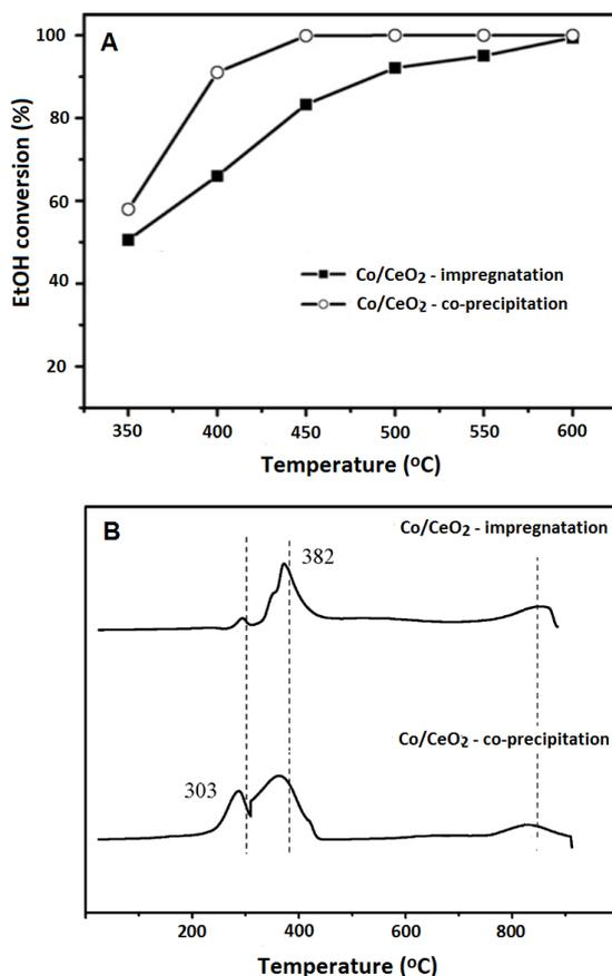
**Fig. 1.11** The ethanol conversion vs. reaction temperature A) and TPR profiles B) for the Co/CeO<sub>2</sub> catalysts prepared via impregnation and co-precipitation techniques. Part of Fig. 4 and Fig. 9 from H. Wang et al. [97] studies.
