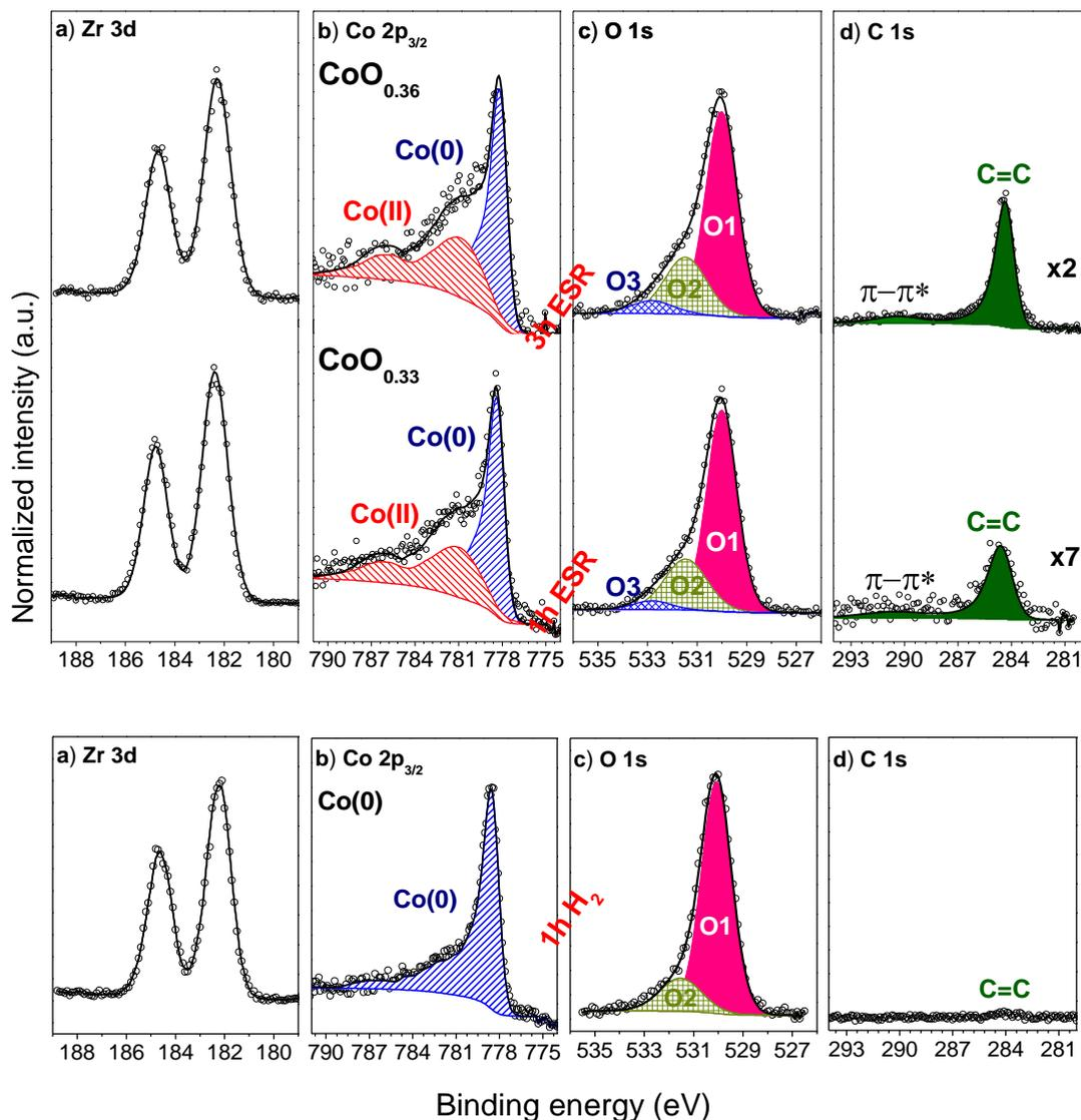
**Fig. 3.** The high resolution XPS spectra of (a) Zr 3d, (b) Co  $2p_{3/2}$ , (c) O 1s and (d) C 1s collected after reduction in hydrogen ( $H_2/Ar$ ,  $420^\circ C$ ), and after the ESR ( $H_2O/EtOH = 12/1$  mol/mol,  $T = 420^\circ C$ ,  $p_{total} = 1$  atm) carried out over the pre-reduced LS-Co/ZrO<sub>2</sub> catalyst; b) Co(II) (▨), Co(0) (▧), c) O1 – lattice oxygen, O2 – hydroxyl and carbonate species, O3 – water.
