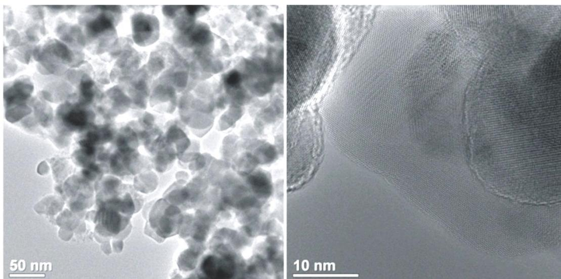
Fig. 8. TEM images of the HS-KCo/ZrO<sub>2</sub> catalyst after 1 h ESR (H<sub>2</sub>O/EtOH = 3/1 mol/mol, 420°C).
