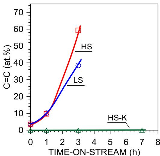
**Fig. 1** The changes of C=C species atomic concentration on the surface of cobalt-based zirconia-supported catalysts versus reaction time of the ESR ( $\text{H}_2\text{O}/\text{EtOH} = 12/1$  mol/mol,  $420^\circ\text{C}$ ,  $p_{\text{total}} = 1$  atm).
