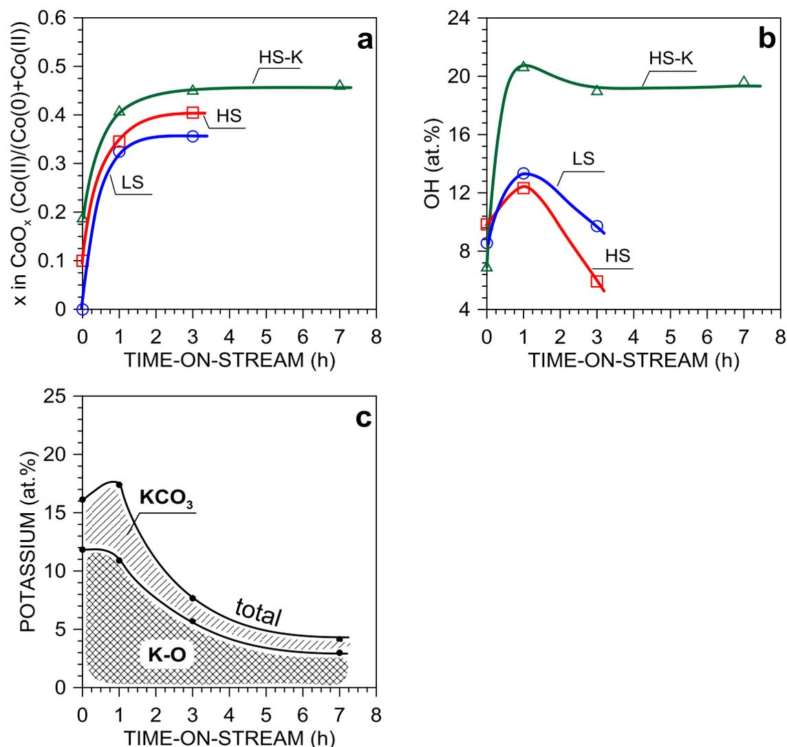
**Fig. 4** The changes of (a) cobalt oxidation state ( $\text{CoO}_x$ ), (b) hydroxyls concentration, (c) potassium containing species, with the time of the ESR ( $\text{H}_2\text{O}/\text{EtOH} = 12/1$  mol/mol,  $420^\circ\text{C}$ ).
