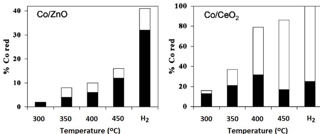
Fig. 1.12 Amount of metallic cobalt in particles dispersion (■) and bigger (□) than the critical diameter obtained after the ESR (300–450°C) and after H<sub>2</sub> treatment at 450°C. Part of Fig 3 from J. Llorca et al. [101].
