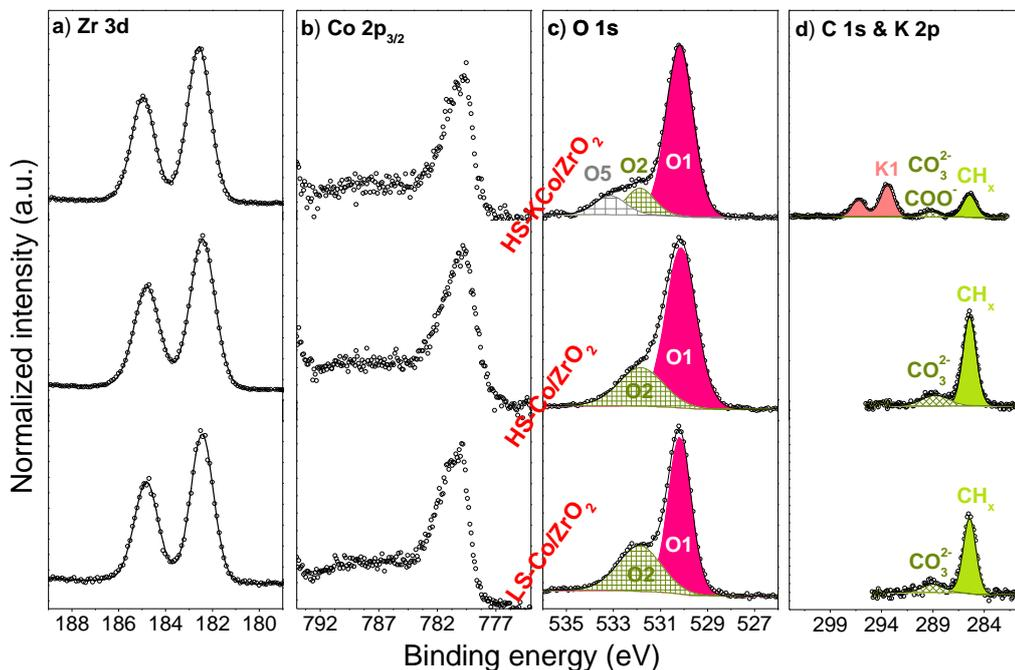
**Fig. S1.** The high resolution XPS spectra of (a) Zr 3d, (b) Co  $2p_{3/2}$ , (c) O 1s and (d) C 1s, Ce 4s & K 2p for fresh (in the oxide form): LS-Co/ZrO<sub>2</sub>, HS-Co/ZrO<sub>2</sub> and HS-KCo/ZrO<sub>2</sub> catalysts; c) O1 – lattice oxygen, O2 – hydroxyl and carbonate species, O5 – COO<sup>-</sup> species d) K1 – KCO<sub>3</sub><sup>2-</sup> and K–O sites.
