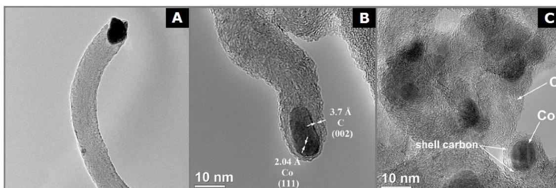
**Fig. 1.25** Chosen TEM images of the KCo/CeO<sub>2</sub> catalyst after 33 h in the ESR at 420°C. A) fiber carbon deposit, B) encapsulating carbon deposit, C) shell carbon encapsulating cobalt particle [140].
