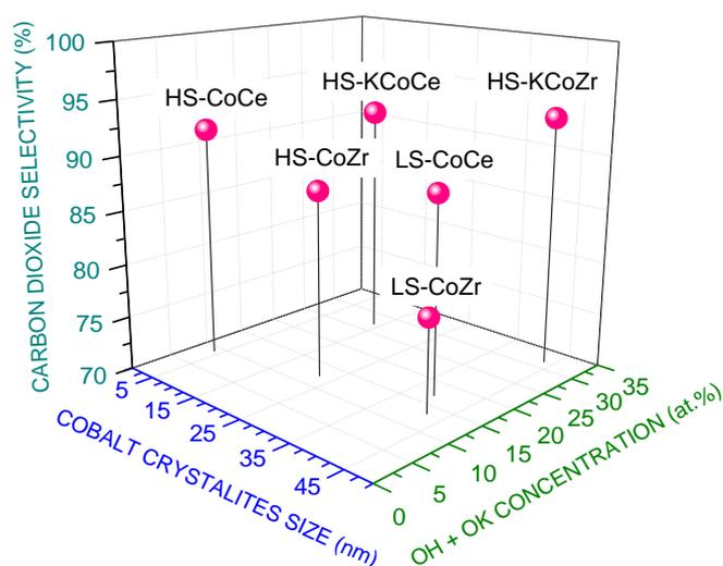
**Fig. 4** The influence of cobalt crystallites size and the surface oxygen-containing species atomic concentration on the ceria- and zirconia-supported catalysts' selectivity towards carbon dioxide ( $H_2O/EtOH = 12/1$  mol/mol,  $420^\circ C$ ,  $t = 1$  h).
