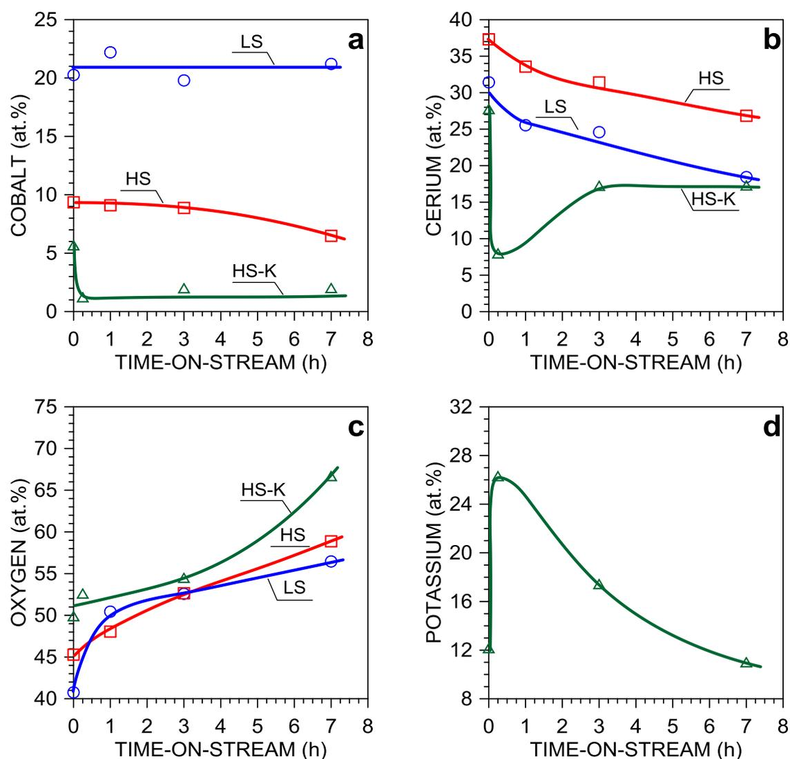
**Fig. 1** The changes of the elemental surface's composition versus reaction time ( $\text{H}_2\text{O}/\text{EtOH} = 12/1$  mol/mol,  $T = 420^\circ\text{C}$ ,  $p_{\text{total}} = 1$  atm). Point "0" on x-axis refers to the composition of the samples pre-reduced in hydrogen ( $420^\circ\text{C}$ ).
