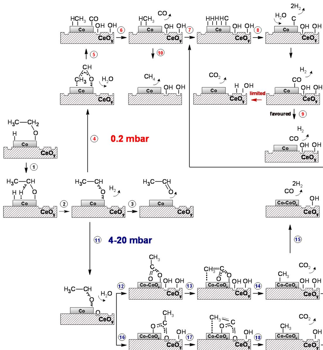
**Fig. 6.** Proposed reaction paths of ESR reaction over Co/CeO<sub>2</sub> catalyst in various pressure regimes. For clarity of the scheme, -OH species adsorbed on cobalt surface are omitted.
