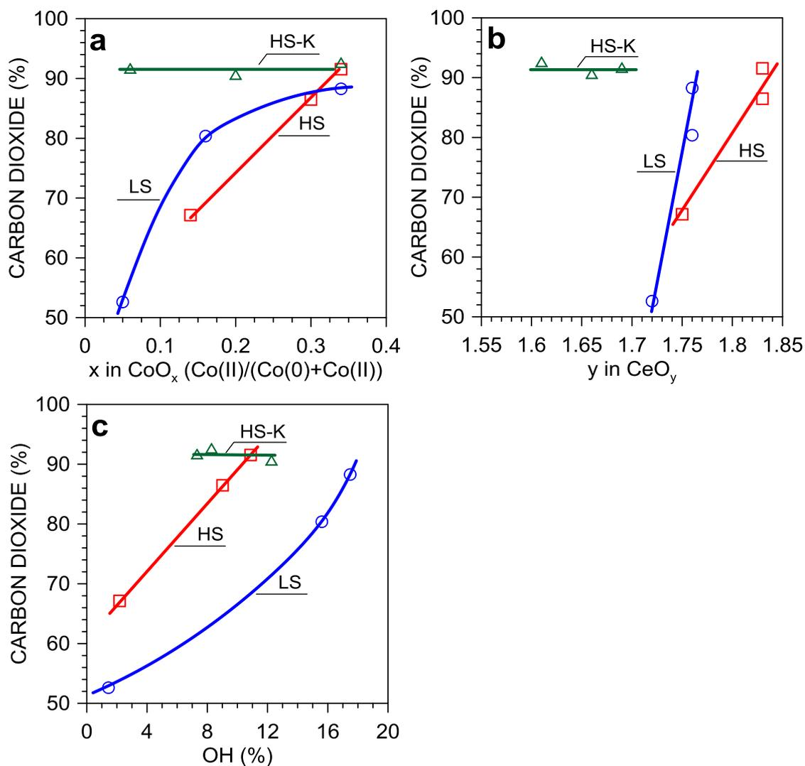
**Figure 11.** Correlation of CO<sub>2</sub> selectivity for the LS-Co/CeO<sub>2</sub>, HS-Co/CeO<sub>2</sub> and HS-KCo/CeO<sub>2</sub> catalysts under the ESR at 420°C with (a) cobalt oxidation state (CoO<sub>x</sub>), (b) ceria valence state (CeO<sub>y</sub>) and (c) percentage contribution of hydroxyls on the surface. Each point represents the different H<sub>2</sub>O/EtOH molar ratio.
