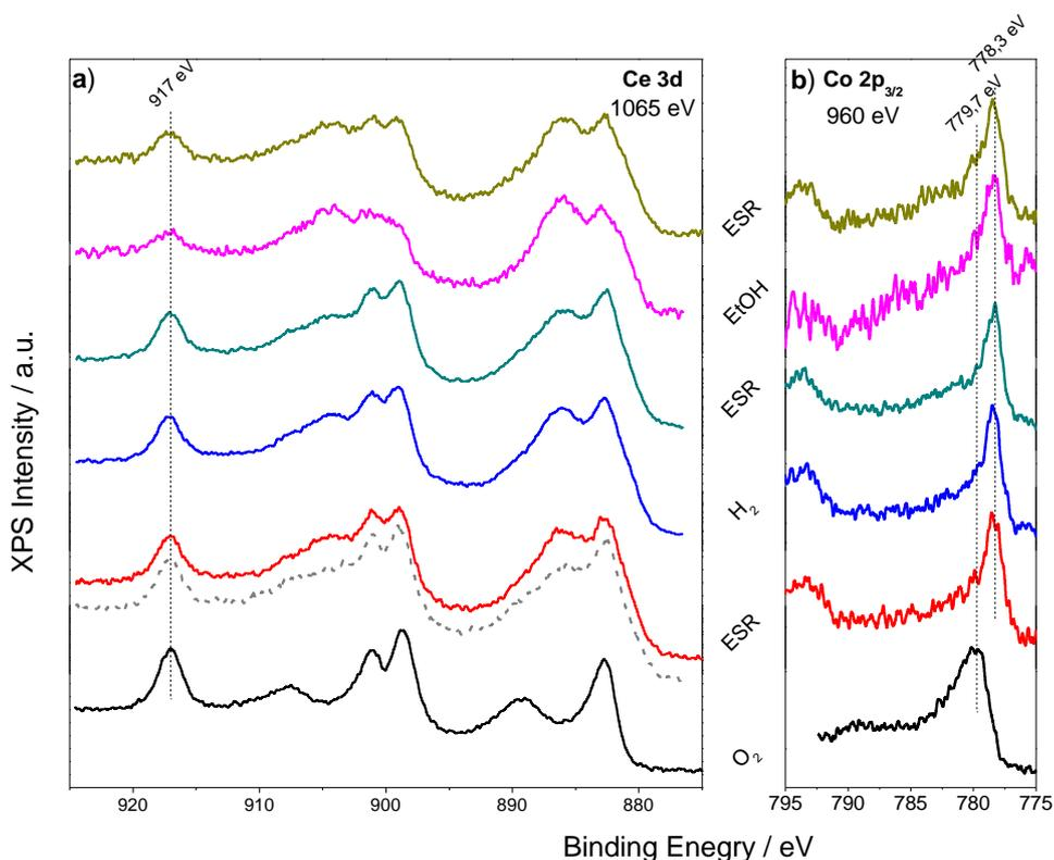
**Fig. 2.** Synchrotron-based XPS (a) Ce 3d ( $h\nu = 1065$  eV) (b) Co  $2p_{3/2}$  ( $h\nu = 960$  eV) spectra of the Co/CeO<sub>2</sub> catalyst in (from bottom to the top): O<sub>2</sub> at 250°C, subsequent ESR reaction (2 experiments with different O<sub>2</sub> pre-treatment duration), H<sub>2</sub> at 420°C, subsequent ESR reaction, EtOH at 420°C, subsequent ESR reaction. The ERS reaction condition were H<sub>2</sub>O/EtOH = 3/1 mol/mol at 420°C and the overall pressure was 0.2 mbar.
