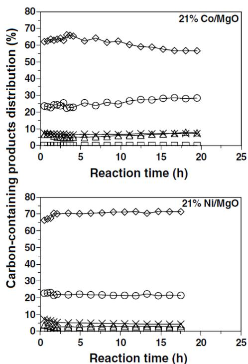
**Fig. 1.5** Product distribution vs. time on stream ( $N_2/H_2O/EtOH = 24/68/8$  vol.%,  $650^\circ C$ ,  $GHSV = 40\,000\ h^{-1}$ ). Part of Fig. 2 from F. Frusteri et al. studies [70]. ( $\diamond$ )  $CO_2$ , ( $\circ$ )  $CO$ , ( $x$ )  $CH_4$ , ( $\Delta$ )  $CH_3CHO$ , ( $\square$ )  $C_2H_4$ .
