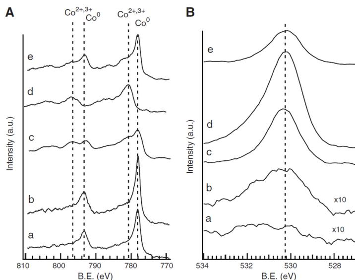
**Fig. 1.15** A) Co 2p and B) O 1s XPS spectra of (a) clean Co foil; (b) Co foil exposed to 60 L  $\text{O}_2$  at  $25^\circ\text{C}$ , (c) Co foil exposed to 9000 L  $\text{O}_2$  at  $730^\circ\text{C}$ , (d) Co foil exposed to  $10^7$  L  $\text{O}_2$  at  $300^\circ\text{C}$ , (e) sample d annealed at  $830^\circ\text{C}$  for 10 min [117].
