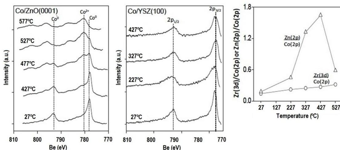
**Fig. 1.17** XPS-spectra of 2 ML Co/ZnO(0001) and Co/YSZ(100) samples as a function of the annealing temperature and Zr 3d/Co 2p and Zn 2p/Co 2p peak area ratios as a function of the sample annealing temperature for both samples. Pictures taken from Ph.D. dissertation of E. Martono [131]. Combined Fig. 3.3 and 5.2.
