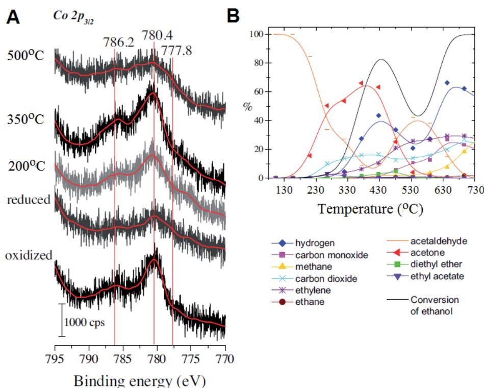
**Fig. 1.18** Co 2p spectra after the ESR at different temperatures on 2%  $\text{Co/CeO}_2$  catalyst A) and selectivities as a function of temperature B). Combined Figs. 2a and 4a from E. Varga et al. studies [123].
