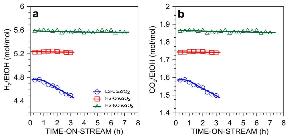
**Fig. 8.** The effect of time-on-stream on (a) hydrogen and (b) carbon dioxide yield obtained over zirconia-supported catalysts ( $\text{H}_2\text{O}/\text{EtOH} = 12/1$  mol/mol,  $420^\circ\text{C}$ ,  $p_{\text{total}} = 1$  atm).
