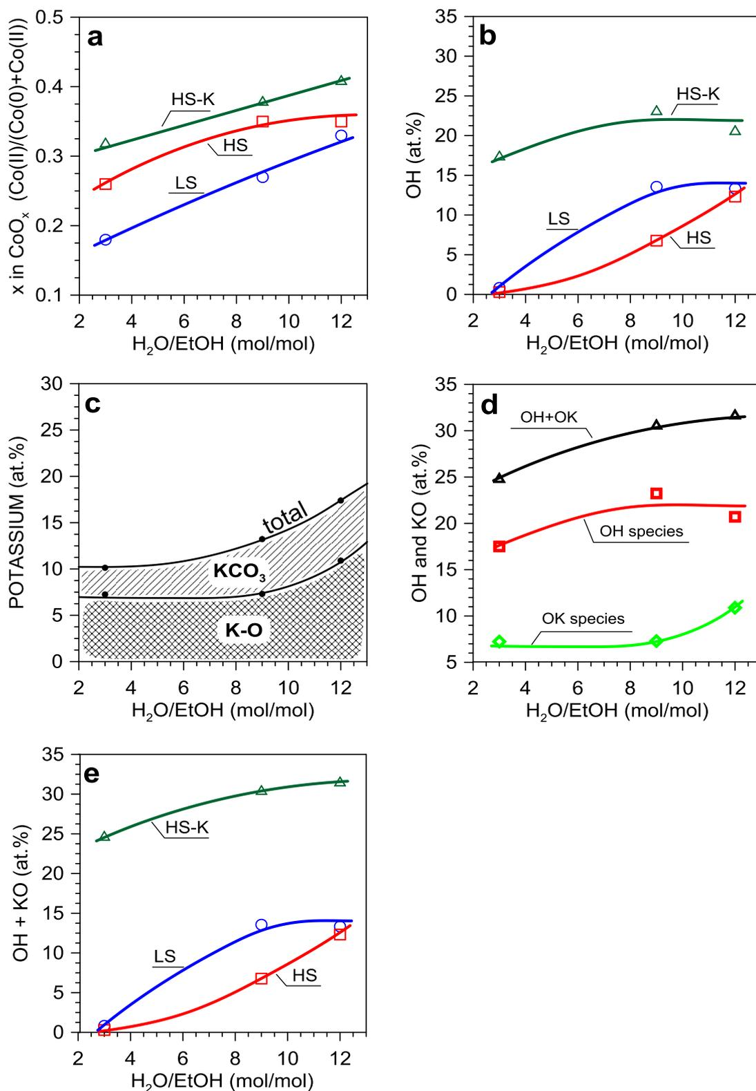
**Fig. 10.** Dependence of (a) cobalt oxidation state ( $CoO_x$ ), (b) percentage concentration of adsorbed hydroxyls, (c) potassium distribution on the catalyst's surface, (d) concentration of OH and K–O sites on HS-K, and (e) concentration of OH + KO sites on the  $H_2O/EtOH$  molar ratio for the LS-Co/ZrO<sub>2</sub>, HS-Co/ZrO<sub>2</sub> and HS-KCo/ZrO<sub>2</sub> catalysts under ESR at 420°C.
