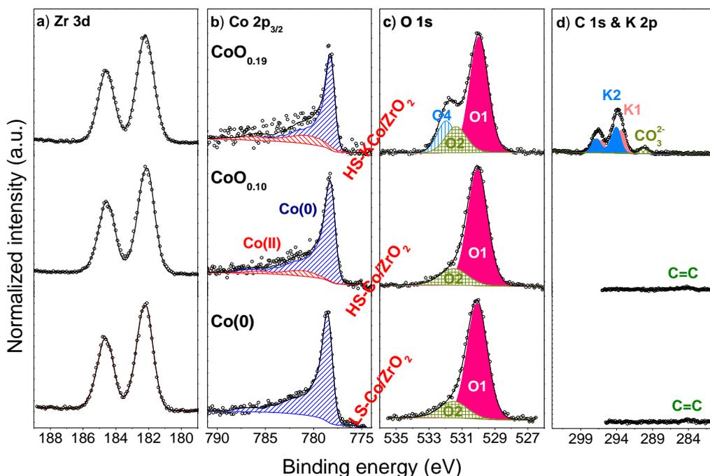
**Fig. 1.** The high resolution XPS spectra of (a) Zr 3d, (b) Co  $2p_{3/2}$ , (c) O 1s and (d) C 1s & K 2p collected after reduction ( $H_2/Ar = 50/50 \text{ cm}^3$ ,  $420^\circ\text{C}$ , 1 h) of LS-Co/ZrO<sub>2</sub>, HS-Co/ZrO<sub>2</sub> and HS-KCo/ZrO<sub>2</sub> catalysts; b) Co(II) (▨), Co(0) (▧), c) O1 – lattice oxygen, O2 – hydroxyl and carbonate species, O4 – carbonate species bonded to potassium, d) probable assignments of K1 and K2 species can be found in the text.
