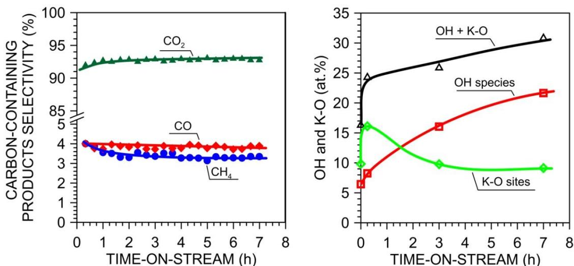
**Fig. 2** The influence of time-on-stream on the ESR selectivity to carbon-containing products and changes of oxygen-containing species concentration on the potassium-promoted nano-ceria-supported catalyst's surface during 7 h in the stream ( $\text{H}_2\text{O}/\text{EtOH} = 12/1$  mol/mol,  $420^\circ\text{C}$ ,  $p_{\text{partial}} = 57$  mbar,  $p_{\text{total}} = 1$  atm).
