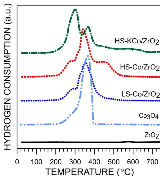
**Fig. 2.** H<sub>2</sub>-TPR profiles of zirconia support, bare cobalt oxide and cobalt-based catalysts.
