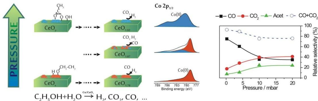
**Fig. 1** The influence of the pressure (0.2–20 mbar) on catalyst's surface state and carbon-containing products distribution (HS-Co/CeO<sub>2</sub>, H<sub>2</sub>O/EtOH=3/1 mol/mol, 420°C).
