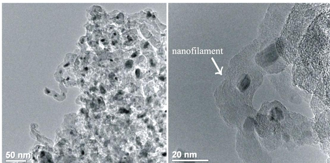
**Fig. 6.** TEM images of the LS-Co/ZrO<sub>2</sub> catalyst after 1 h ESR (H<sub>2</sub>O/EtOH =3/1 mol/mol, 420°C).
