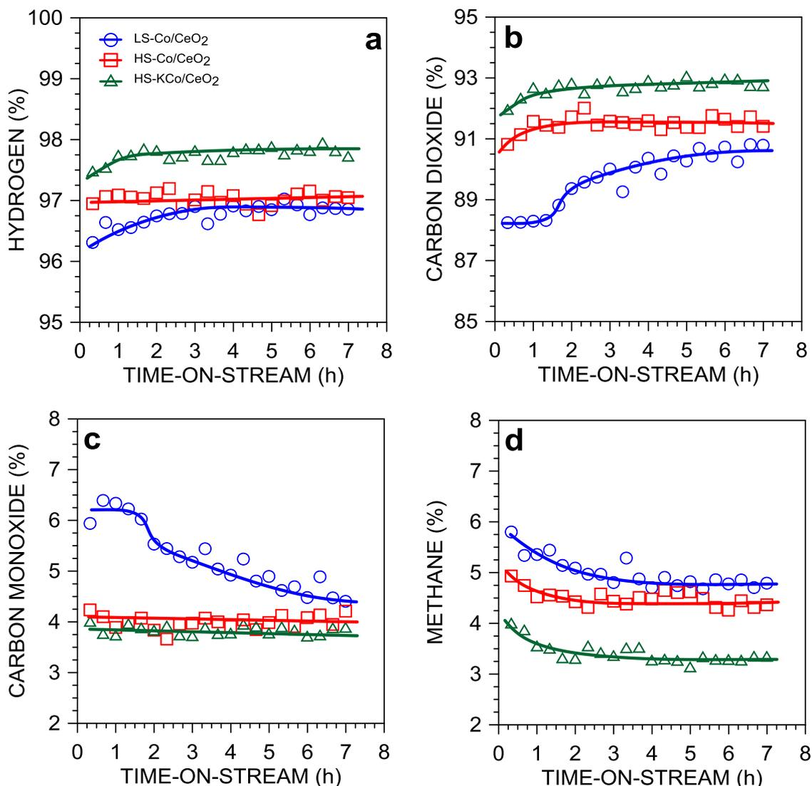
**Fig. 6.** The effect of time-on-stream on ceria-supported catalysts' selectivity towards hydrogen, carbon dioxide, carbon monoxide and methane ( $\text{H}_2\text{O}/\text{EtOH} = 12/1$  mol/mol,  $420^\circ\text{C}$ ,  $p_{\text{total}} = 1$  atm).
