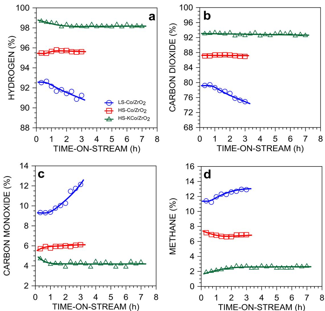
**Fig. 7.** The effect of time-on-stream on zirconia-supported catalysts' selectivity towards hydrogen, carbon dioxide, carbon monoxide and methane ( $\text{H}_2\text{O}/\text{EtOH} = 12/1$  mol/mol,  $420^\circ\text{C}$ ,  $p_{\text{total}} = 1$  atm).
