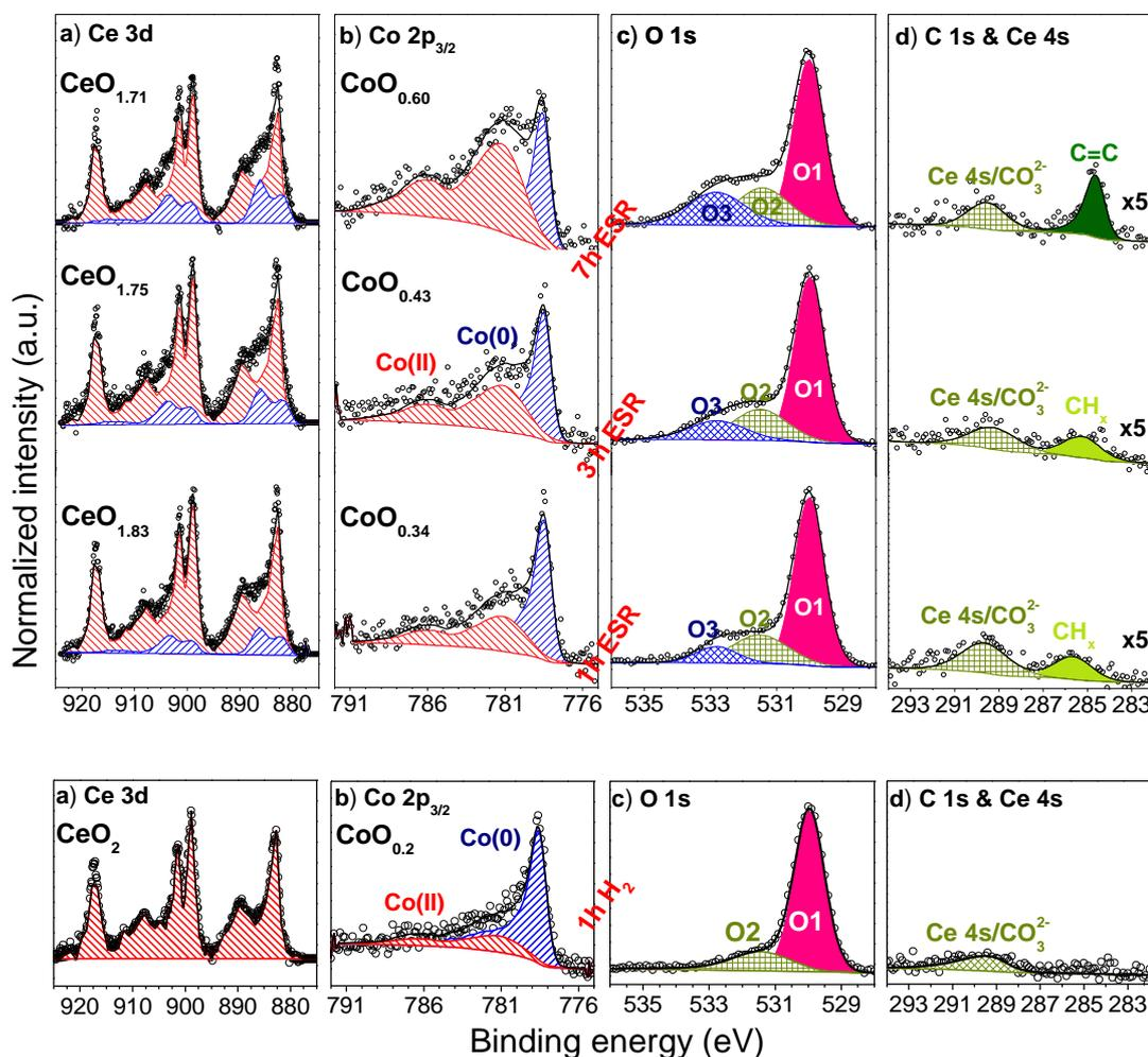
**Fig. 4.** The high resolution XPS spectra of (a) Ce 3d, (b) Co 2p<sub>3/2</sub>, (c) O 1s and (d) C 1s & Ce 4s collected after reduction in hydrogen (H<sub>2</sub>/Ar, 420°C), and after the ESR (H<sub>2</sub>O/EtOH = 12/1 mol/mol, T = 420°C, p<sub>total</sub> = 1 atm) carried out over the pre-reduced (H<sub>2</sub>/Ar, T = 420°C) HS-Co/CeO<sub>2</sub> catalyst; a) Ce(IV) (///), Ce(III) (///), b) Co(II) (///), Co(0) (///), c) O1 – lattice oxygen, O2 – hydroxyl and carbonate species, O3 – water.
