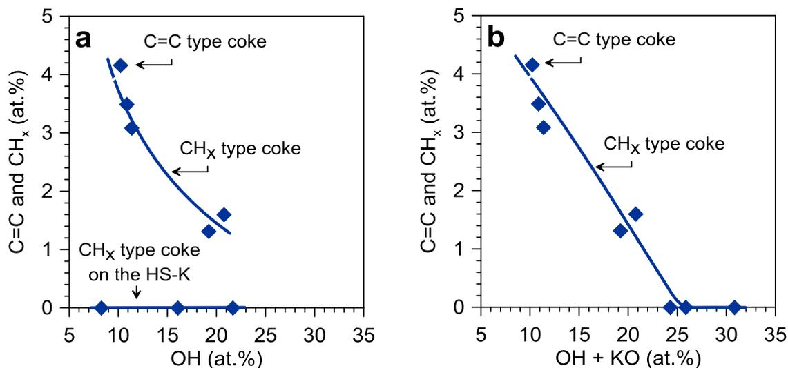
**Fig. 9** Correlation of atomic percentage contribution of C=C and CH<sub>x</sub> species with (a) hydroxyls concentration, and (b) sum of hydroxyls and K–O sites on the catalysts' surface.
