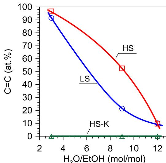
**Fig. 9.** Dependence of percentage contribution of C=C species on the catalysts' surface, on the H<sub>2</sub>O/EtOH molar ratio for the LS-Co/ZrO<sub>2</sub>, HS-Co/ZrO<sub>2</sub> and HS-KCo/ZrO<sub>2</sub> catalysts under ESR at 420°C.
