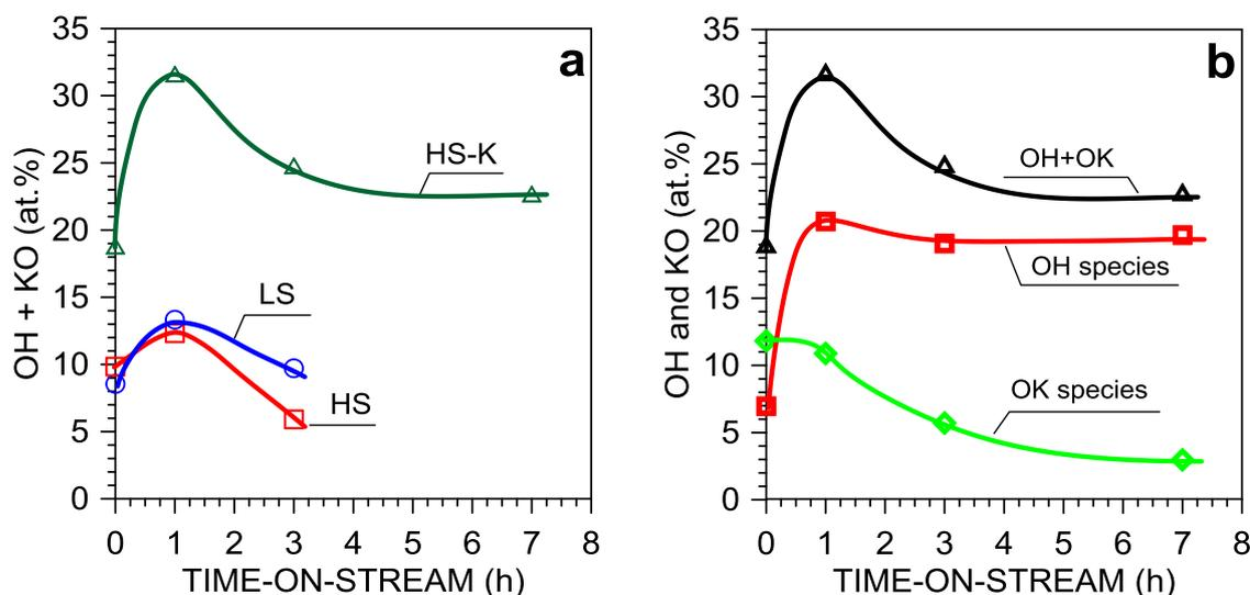
**Fig. 9** The changes of hydroxyls and K–O sites with time-on-stream ( $\text{H}_2\text{O}/\text{EtOH} = 12/1$  mol/mol,  $420^\circ\text{C}$ ) for (a) zirconia-supported cobalt catalysts and (b) HS-K catalyst.
