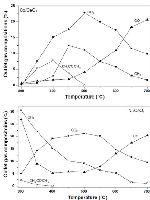
**Fig. 1.8** Effect of the reaction temperature on products distribution over Co/CeO<sub>2</sub> and Ni/CeO<sub>2</sub> catalysts for the H<sub>2</sub>O/EtOH = 3/1 mol/mol. Part of Fig. 5 from B. Zhang et al. studies [20].
