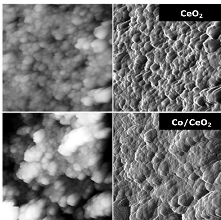
**Fig S2.1.** AFM images of CeO<sub>2</sub> (top), Co/CeO<sub>2</sub> catalyst (bottom) (side of the picture is 1  $\mu$ m).
