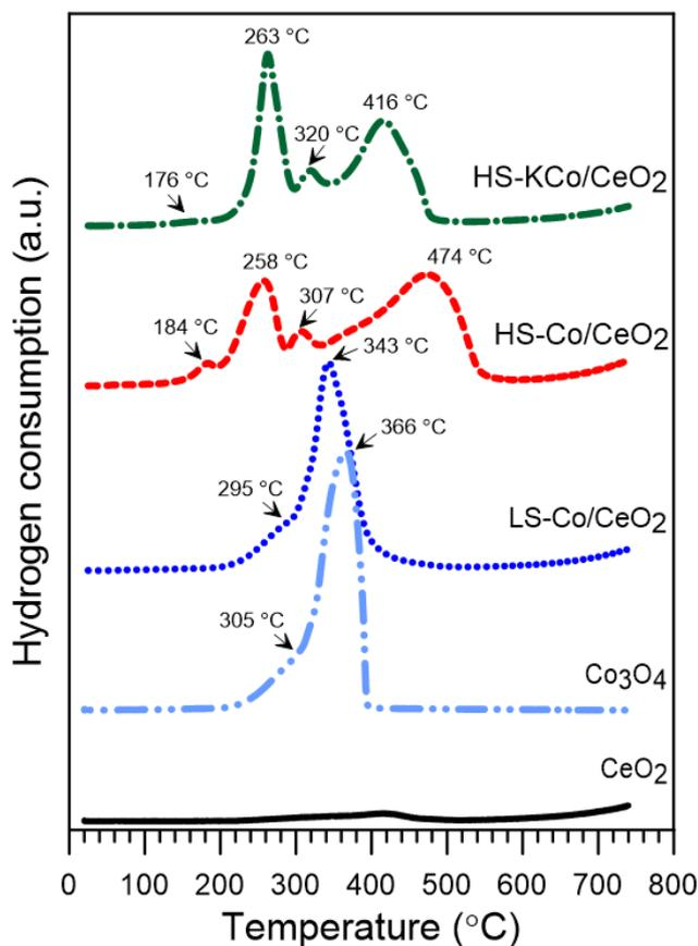
**Figure 1.** H<sub>2</sub>-TPR profiles of as calcined ceria support, Co<sub>3</sub>O<sub>4</sub> and cobalt-based catalysts.
