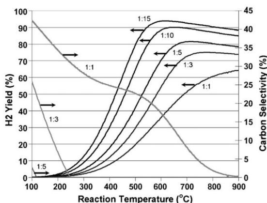
**Fig. 1.2** Effect of  $\text{H}_2\text{O}/\text{EtOH}$  molar ratio on equilibrium hydrogen yield and carbon selectivity (no dilution) [4].
