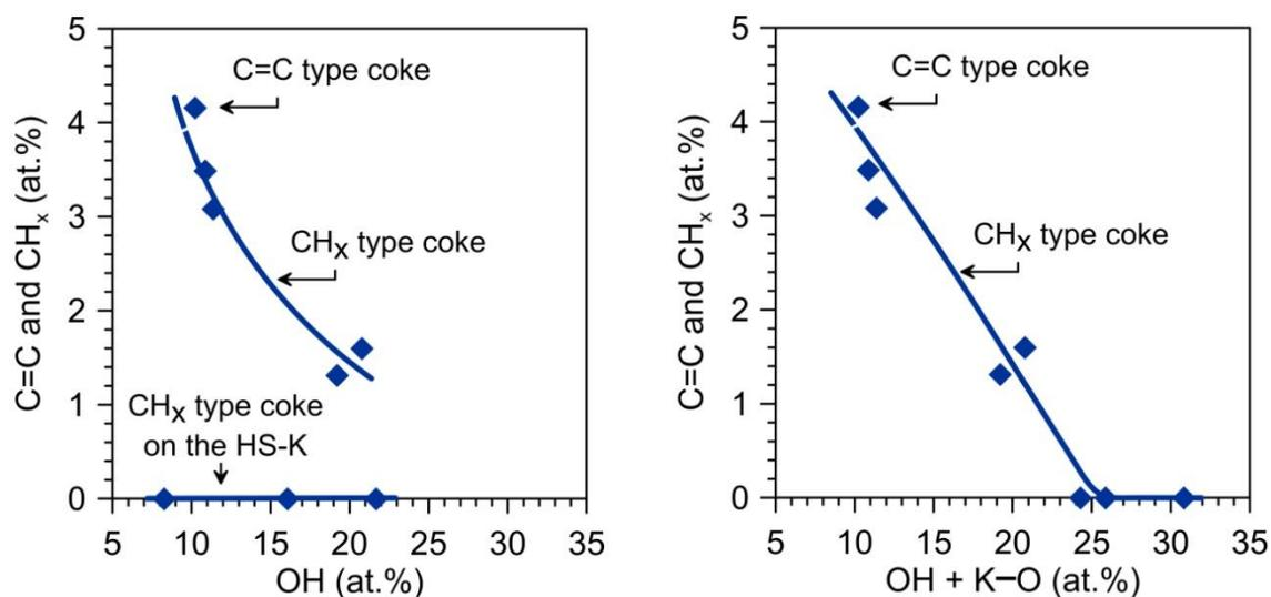
**Fig. 3** Correlation of atomic percentage contribution of C=C and  $\text{CH}_x$  species with hydroxyls concentration, and sum of hydroxyls and K–O sites on the ceria-supported cobalt catalysts' surface.
