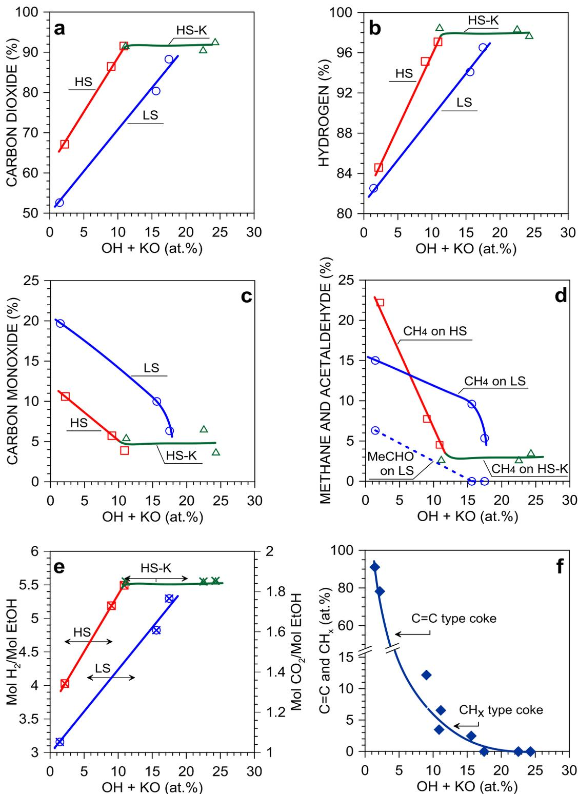
**Figure 12.** Correlation of (a–d) the catalysts selectivity towards H<sub>2</sub> and carbon-containing product, (e) H<sub>2</sub> and CO<sub>2</sub> yield, and (f) the concentration of C=C and CH<sub>x</sub> species on the whole surface, with the concentration of oxygen-containing species on the surface of the LS-Co/CeO<sub>2</sub>, HS-Co/CeO<sub>2</sub> and HS-KCo/CeO<sub>2</sub> catalysts under the ESR at 420°C.
