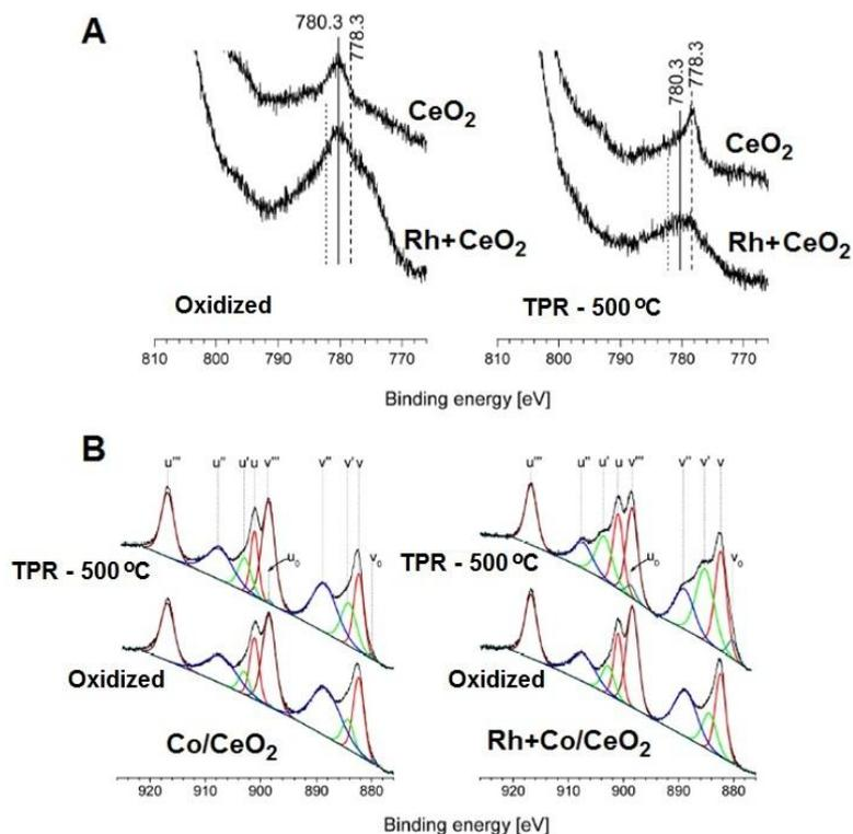
**Fig. 1.19** A) Co 2p XPS spectra on ceria support after oxidation at 400°C for 30 min and after linear heating (20°C/min) in H<sub>2</sub> to 500°C, B) Ce 3d XPS spectra taken on a 2% Co/CeO<sub>2</sub> catalyst and 0.1% Rh + 2% Co/CeO<sub>2</sub> catalyst after oxidation at 400°C and after reduction with the TPR run up to 500°C. Part of Fig. 2 from Zs. Ferencz et al. studies [124].
