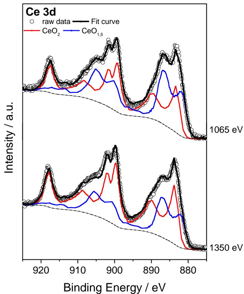
**Fig. SI4** Example of Ce 3d spectra deconvolution using Ce 3d components recorded on reference samples. Spectra recorded using different photon energies are shown. Please note the relatively higher CeO<sub>1,5</sub> component at the spectrum recorded using 1065 photon energy.
