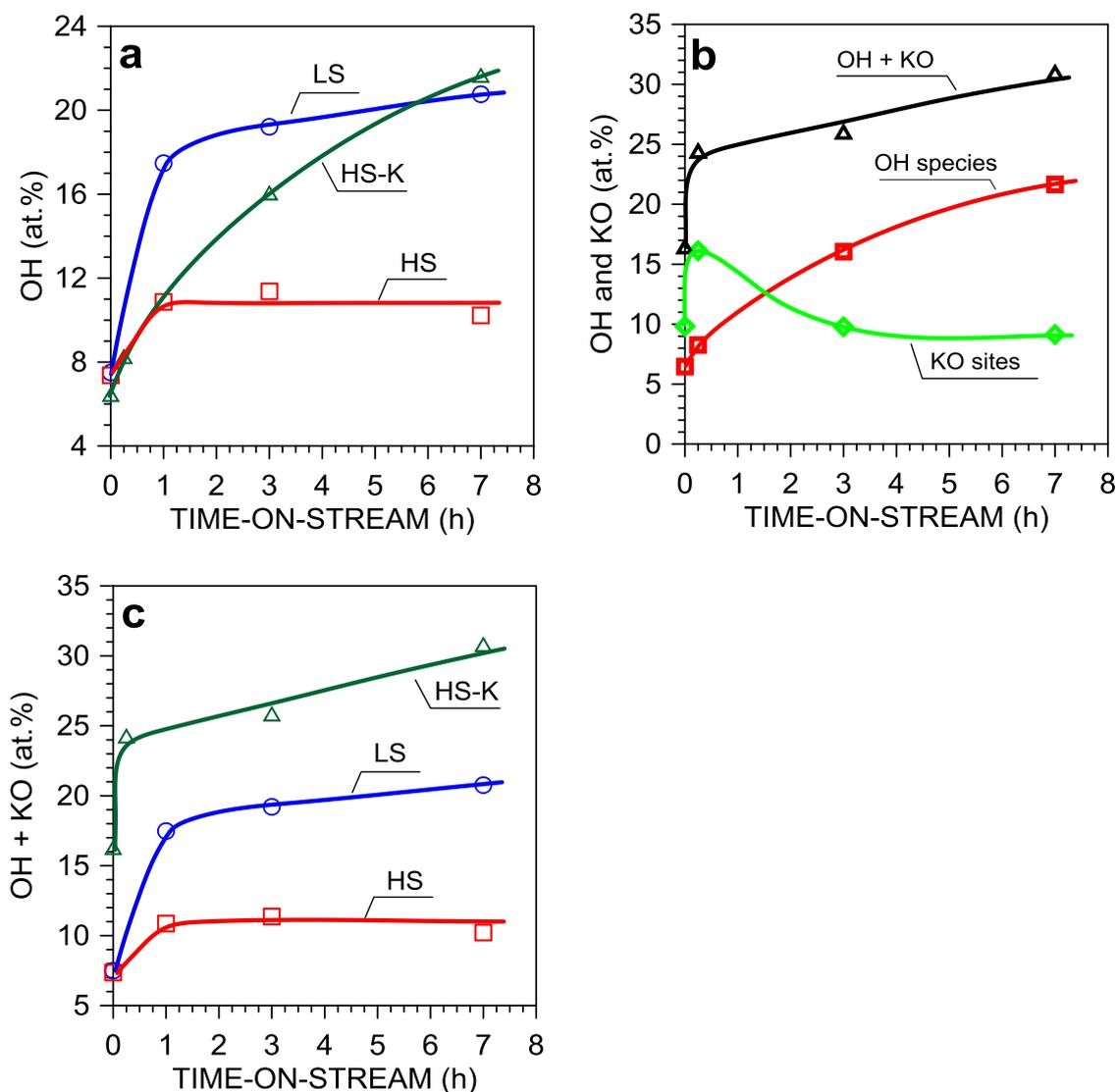
**Fig. 8** The changes of hydroxyls and K–O sites with time-on-stream (H<sub>2</sub>O/EtOH = 12/1 mol/mol, 420°C) for ceria-supported cobalt catalysts.
