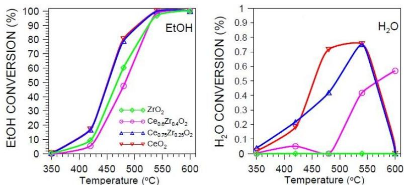
**Fig. 1.22** Conversion of ethanol and water at temperatures 350–600°C over high-surface area ceria, zirconia and binary ceria-zirconia oxides [174].
