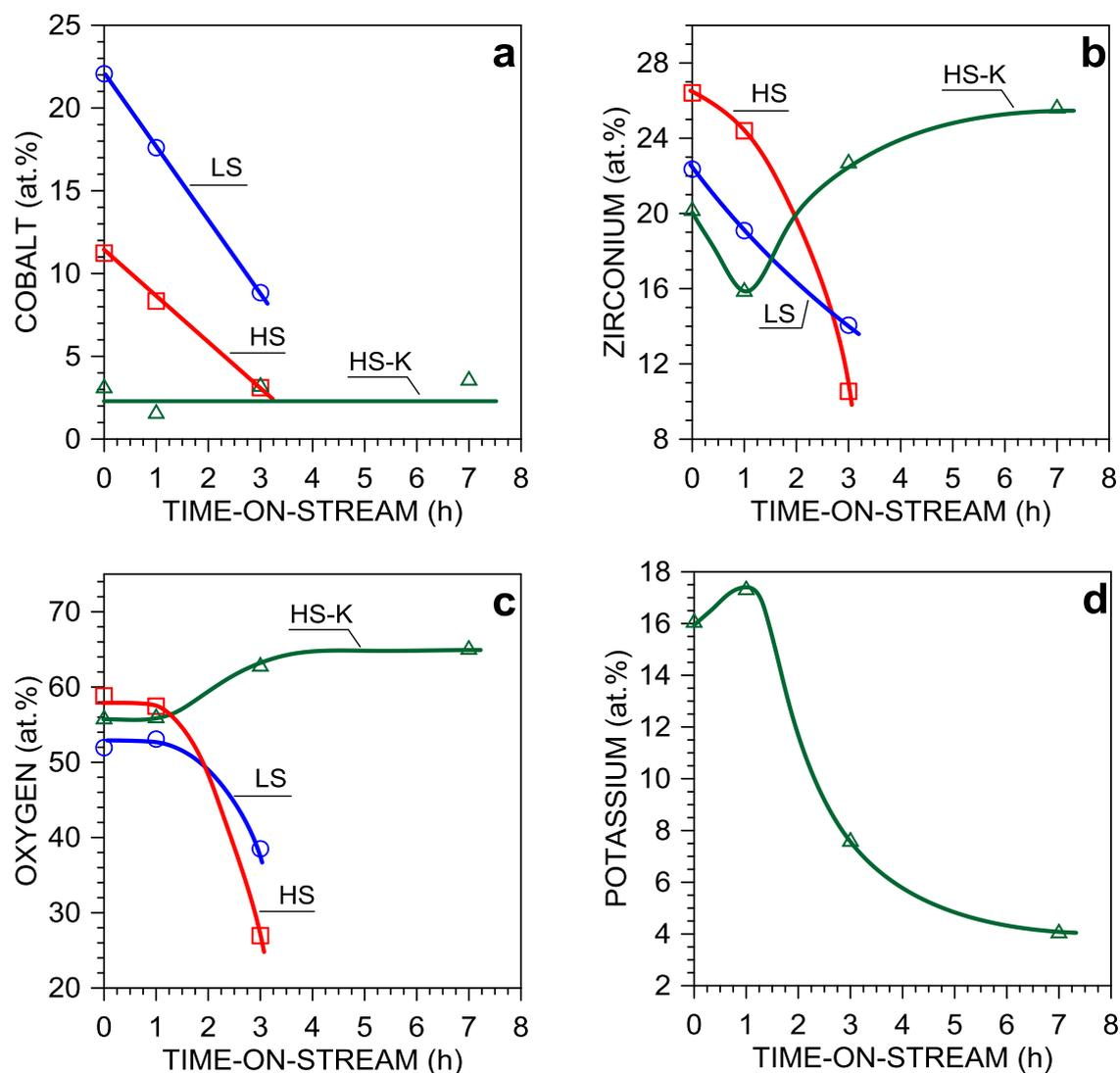
**Fig. 2** The changes of elemental surface's composition of cobalt-based zirconia-supported catalysts with the ESR reaction time ( $\text{H}_2\text{O}/\text{EtOH} = 12/1$  mol/mol,  $420^\circ\text{C}$ ,  $p_{\text{total}} = 1$  atm).
