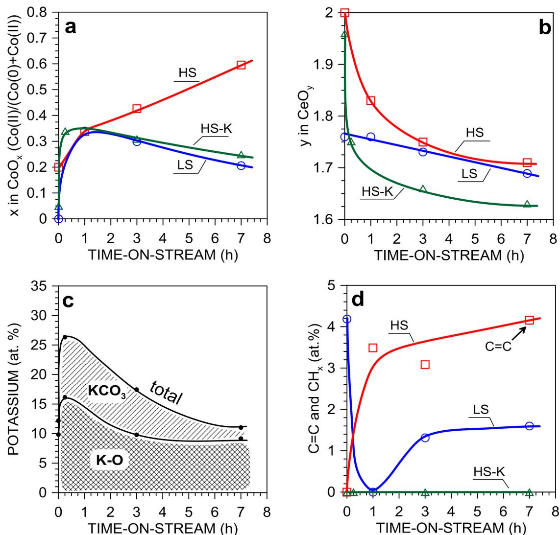
**Fig. 3** The changes of (a) cobalt oxidation state (CoO<sub>x</sub>), (b) ceria valence state (CeO<sub>y</sub>), (c) potassium-containing species, (d) amount of C=C and CH<sub>x</sub> species, with the reaction time (H<sub>2</sub>O/EtOH = 12/1 mol/mol, 420°C).
