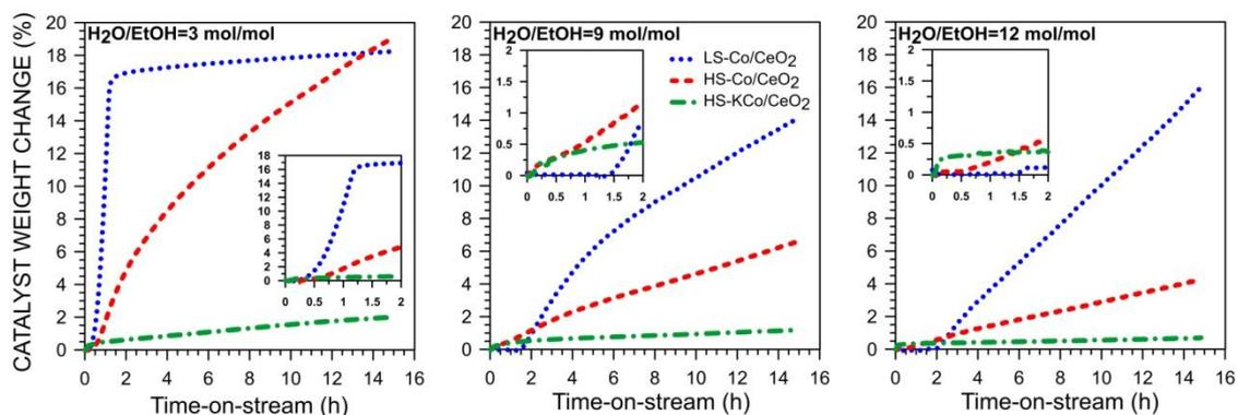
**Figure 6.** The gravimetric results for the LS-Co/CeO<sub>2</sub> (···), HS-Co/CeO<sub>2</sub> (---) and HS-KCo/CeO<sub>2</sub> (- · -) catalysts under the H<sub>2</sub>O/EtOH = 3/1, 9/1 and 12/1 mol/mol.
