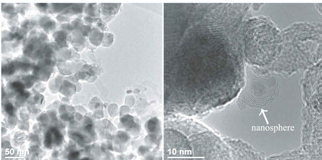
**Fig. 7.** TEM images of the HS-Co/ZrO<sub>2</sub> catalyst after 1 h ESR (H<sub>2</sub>O/EtOH =3/1 mol/mol, 420°C).
