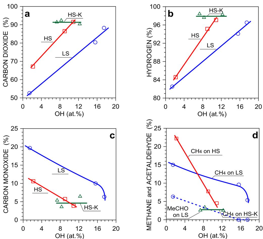
**S. 2** Correlation of (a–d) the catalysts' selectivity towards H<sub>2</sub> and carbon-containing product with the concentration of hydroxyls on the surface of the LS-Co/CeO<sub>2</sub>, HS-Co/CeO<sub>2</sub> and HS-KCo/CeO<sub>2</sub> catalysts under the ESR at 420°C.
