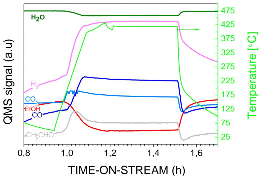
**Fig. SI5.** Characteristic *on-line* mass spectrometry data (after fragment correction) recorded upon heating the Co/CeO<sub>2</sub> catalyst in the ESR reaction mixture (EtOH/H<sub>2</sub>O = 1/3 mol/mol, 420°C, 0.2 mbar). The green line is the sample temperature corresponding to the right y-axis.
