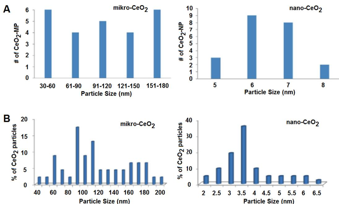
**Fig. 1.10** Particle size distribution histograms of the micro- and nano-Co/CeO<sub>2</sub>. Combined figures from the studies of I.I. Soykal et. al A) [80] (Fig. 1) and B) [79] (Fig. 3).
