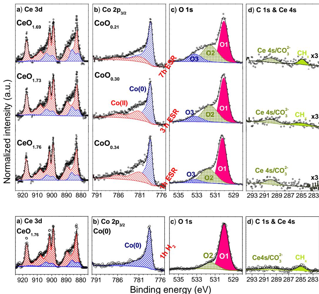
**Fig. 2.** The high resolution XPS spectra of (a) Ce 3d, (b) Co 2p<sub>3/2</sub>, (c) O 1s and (d) C 1s & Ce 4s collected after reduction in hydrogen (H<sub>2</sub>/Ar, 420°C), and after the ESR (H<sub>2</sub>O/EtOH = 12/1 mol/mol, T = 420°C, p<sub>total</sub> = 1 atm) carried out over the pre-reduced LS-Co/CeO<sub>2</sub> catalyst; a) Ce(IV) (///), Ce(III) (///), b) Co(II) (///), Co(0) (///), c) O1 – lattice oxygen, O2 – hydroxyl and carbonate species, O3 – water.
