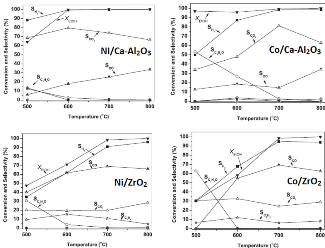
**Fig. 1.7** Effect of reaction temperature on ethanol conversion and product selectivities over nickel- and cobalt-based Ca- $\gamma$ -Al<sub>2</sub>O<sub>3</sub> and ZrO<sub>2</sub> supported catalysts. Based on Fig. 5 and 6 from L. Chen et al. studies [28].
