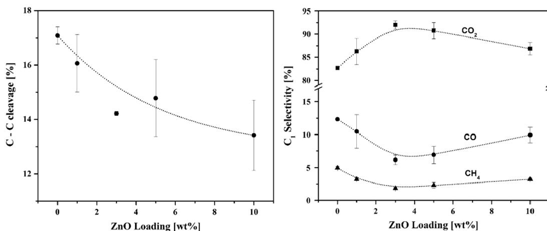
**Fig. 1.21** The C–C cleavage conversion and C<sub>1</sub>-products selectivity for different zinc oxide loading in the cobalt catalysts. Combined Fig. 6 and 7 from S. Davidson et al. studies [157].
