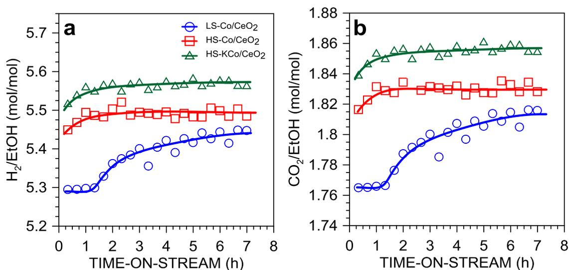
**Fig. 7.** The effect of time-on-stream on hydrogen (a) and carbon dioxide (b) yield for ceria-supported catalysts (H<sub>2</sub>O/EtOH = 12/1 mol/mol, 420°C, p<sub>total</sub> = 1 atm).
