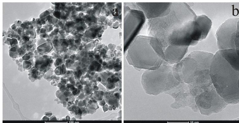
**Figure 9.** TEM images of the HS-KCo/CeO<sub>2</sub> catalyst after 1 h ESR ( $T = 420^{\circ}\text{C}$ ,  $\text{H}_2\text{O}/\text{EtOH} = 3/1$  mol/mol).
