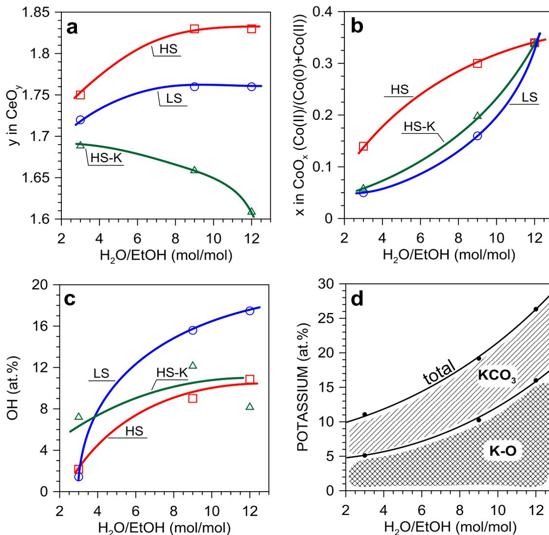
**Figure 10.** Dependence of (a) ceria valence state ( $\text{CeO}_y$ ), (b) cobalt oxidation state ( $\text{CoO}_x$ ), (c) percentage concentration of adsorbed hydroxyls, and (d) potassium distribution on the catalyst surface, with the  $\text{H}_2\text{O}/\text{EtOH}$  molar ratio for the LS-Co/ $\text{CeO}_2$ , HS-Co/ $\text{CeO}_2$  and HS-KCo/ $\text{CeO}_2$  catalysts under ESR at  $420^\circ\text{C}$ .
