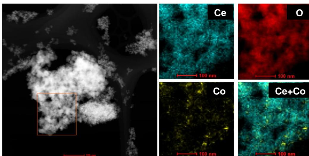
**Fig. 1.** STEM image with selected area mapping and STEM-EDS spectrum images showing the elemental composition of calcined Co/CeO<sub>2</sub> catalysts.
