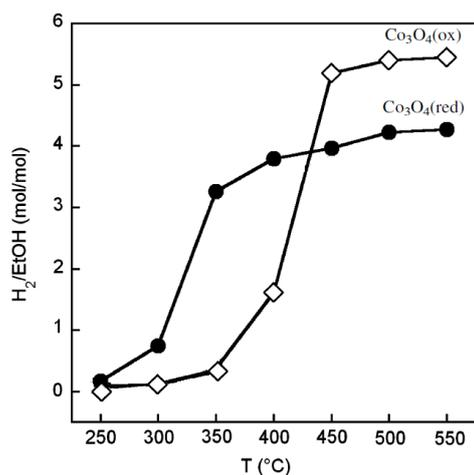
**Fig. 1.14** Efficiency of ethanol steam reforming over the pre-oxidized and the pre-reduced  $\text{Co}_3\text{O}_4$  under the  $\text{H}_2\text{O}/\text{EtOH} = 3.5/1$  mol/mol carried out at 250–550°C. Part of Fig. 3 from studies of S. Tuti and F. Pepe [19].
