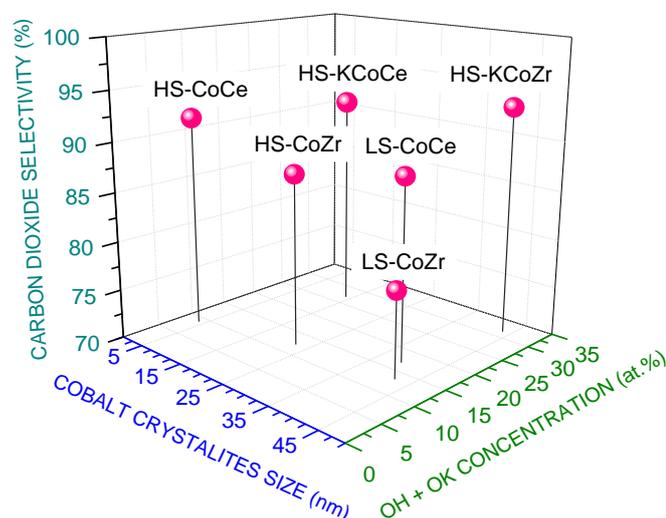
**Fig. 5** The influence of cobalt crystallites size and the surface oxygen-containing species atomic concentration on the ceria- and zirconia-supported catalysts' selectivity towards carbon dioxide (H<sub>2</sub>O/EtOH = 12/1 mol/mol, 420°C, t = 1 h).
