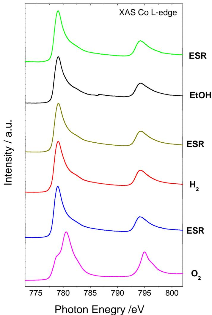
**Fig. S3.** Total electron yield (TEY) mode Co L-edge XAS spectra of Co/CeO<sub>2</sub> catalysts recorded at conditions the same conditions with the Co 2p<sub>3/2</sub> XPS spectra presented in Fig. 2 in the main text. Namely (from bottom to the top) 0.2 mbar of O<sub>2</sub> at 250°C, subsequent ESR reaction (H<sub>2</sub>O/EtOH = 3/1 mol/mol) at 420°C, 0.2 mbar of H<sub>2</sub> at 420°C, subsequent ESR reaction, 0.2 mbar of EtOH at 420°C, subsequent ESR reaction.
