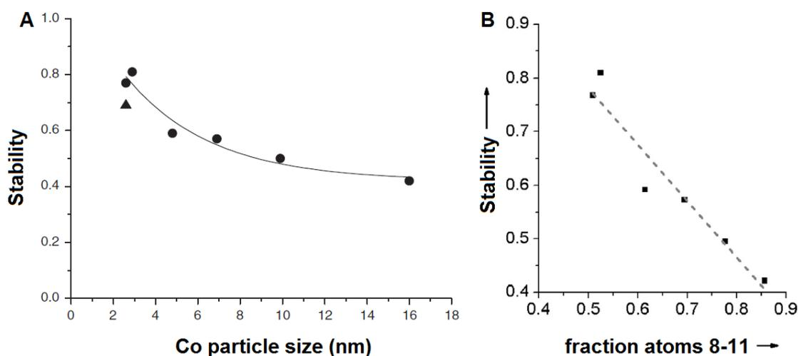
**Fig. 1.9** Stability of Co/CNF A) as a function of cobalt particle size ( $\text{EtOH}/\text{H}_2\text{O} = 1/3$  mol/mol,  $500^\circ\text{C}$ ), B) as a function of the fraction of surface atoms with coordination number 8–11, like in terraces. Combined Fig. 3 and 6b from A.L.M. da Silva et al. studies [82].
