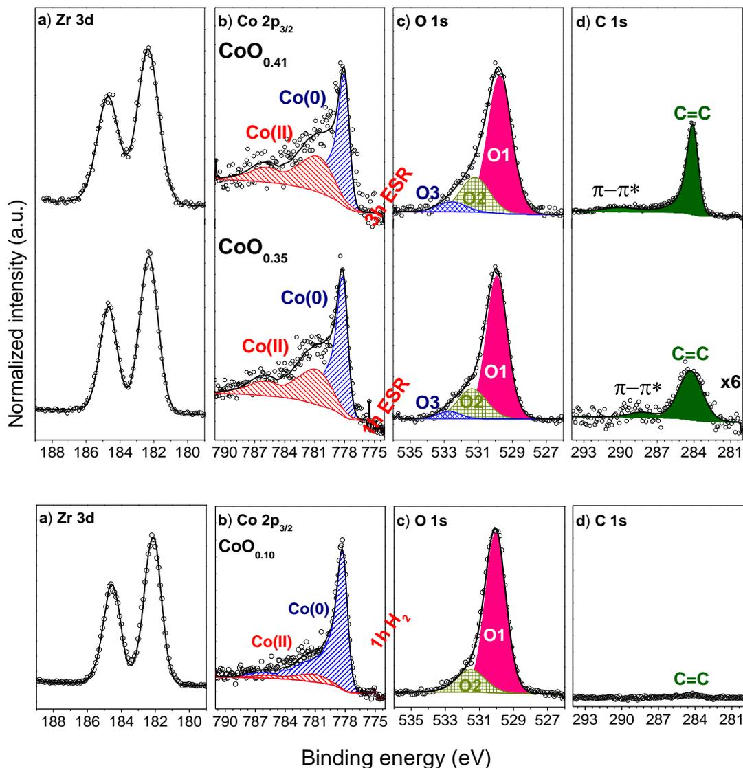
**Fig. 5.** The high resolution XPS spectra of (a) Zr 3d, (b) Co  $2p_{3/2}$ , (c) O 1s and (d) C 1s collected after reduction in hydrogen ( $H_2/Ar$ ,  $420^\circ C$ ), and after the ESR ( $H_2O/EtOH = 12/1$  mol/mol,  $T = 420^\circ C$ ,  $p_{total} = 1$  atm) carried out over the pre-reduced ( $H_2/Ar$ ,  $T = 420^\circ C$ ) HS-Co/ZrO<sub>2</sub> catalyst, b) Co(II) (///), Co(0) (////), c) O1 – lattice oxygen, O2 – hydroxyl and carbonate species, O3 – water.
