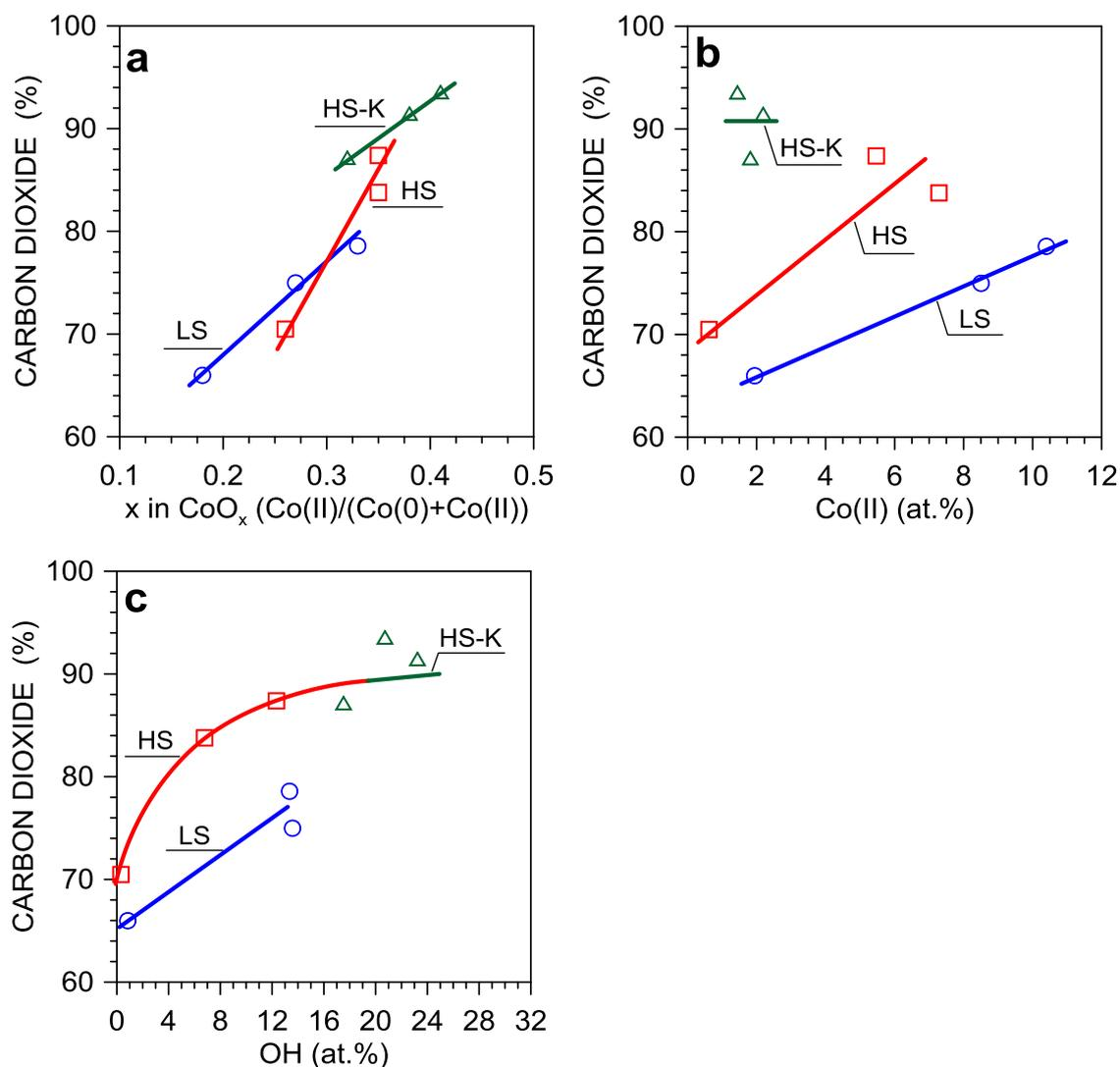
**Fig. 11.** Correlation of CO<sub>2</sub> selectivity for the LS-, HS- and HS-K catalysts under the ESR at 420°C with (a) cobalt oxidation state (CoO<sub>x</sub>), (b) cobalt ions Co(II) surface atomic concentration, and (c) percentage contribution of hydroxyls on the surface.
