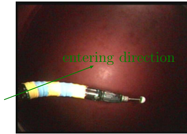
Figure 4.8: The green line represent the estimated instrument entering direction. The first yellow marker encountered walking along this line is considered to be the root (i.e. the first marker) of the tree.
