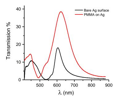
**Figure 3.10:** The zero-order transmission spectra at normal incidence for a hexagonal hole-array ( $a_0 = 380$  nm) before (black curve) and after (red curve) the deposition of a 100 nm layer of PMMA on its surface.
