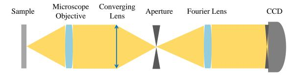
**Figure 4.7:** Detection scheme of the home built set up used for dispersion measurements showing the passage of light coming out of the sample through main parts of the set up.
