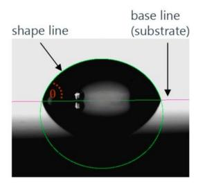
**Figure 3.20:** Image of a sessile drop taken by the DSA100 instrument with its fitted contour (shown in green). The figure is reproduced from (<a href="https://www.kruss.de/services/education-theory/glossary/drop-shape-analysis/">https://www.kruss.de/services/education-theory/glossary/drop-shape-analysis/</a>)
