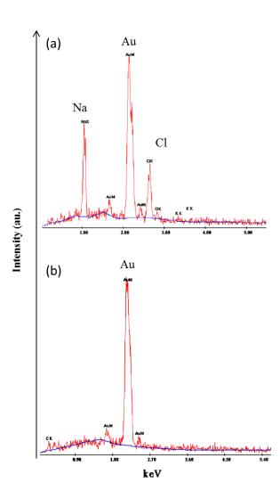
**Figure 3.28:** EDX analysis spectra showing the elemental analysis on sample of Figure 3.25 (a) when probing the features (b) when probing the Au surface away from features. The blue curve represents the background signal.
