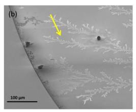
**Figure 3.26:** SEM image of the feature present in Figure 3.25 due to the water droplet. (a) The whole feature showing a contrast at the circumference. (b) A magnified SEM image of the area pointed by yellow arrow in (a).
