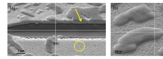
**Figure 3.27:** SEM images: (a) at 23K times magnification and shows the cross cut at the features. A clear contrast between the original Au film and the features is pointed by the yellow arrow. (b) At 90K times magnification, showing the area inside the yellow circle of (a) and highlighting the roughness modification to the surface imposed by the features.
