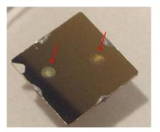
**Figure 3.25:** Captured photo for the Au sample showing the features (indicated by the red arrows) left after the evaporation of triple distilled water droplets.
