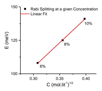
**Figure 4.9:** Variation of the Rabi splitting as a function of the square root of Ce6 concentration in DMF. The black squares are the Rabi splitting value corresponding to each concentration (6%, 8%, and 10% in weight in DMF), and the red line is their linear fit.
