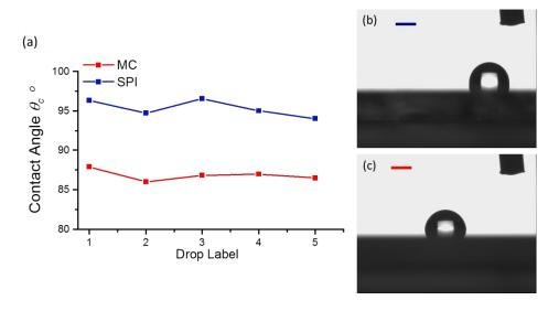
**Figure 3.22:** (a) The value of contact angle measured for a set of 5 different drops on the surface of (b) SPI before and (c) after irradiation with UV.
