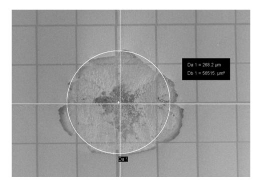
Figure 3.24: SEM image on a section of the large array showing the mark left by the water droplet (having an area of  $\sim 56515 \ \mu m^2$ ) after its evaporation.
