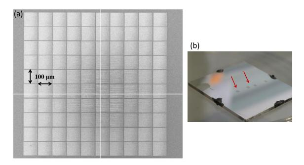
**Figure 3.21:** (a) SEM image of a  $\sim$  1 mm<sup>2</sup> large plasmonic array milled in 120 nm Ag film by using Auriga FIB machine. The small squares are identical hexagonal hole-arrays ( $a_0 = 250$  nm, D = 120 nm) separated by 5  $\mu$ m from each side. (b) A captured photo for the sample carrying arrays different periodicities indicated by the red arrows.
