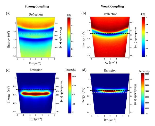
**Figure 4.10:** Angle resolved dispersion reflection spectra from high concentration (strong coupling regime) (a) and low concentration (weak coupling regime) (b) Ce6/DMF solution-filled cavities resonant with the Ce6 transition energy (dashed lines). The emission dispersion curves from the same cavities are shown in (c) and (d) with normal incidence excitation at 532 nm.
