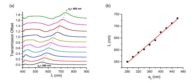
**Figure 3.8:** (a) The zero-order transmission spectra at normal incidence of hexagonal hole-arrays with varying periodicities (a<sub>0</sub>) from 280 nm to 460 nm milled in Ag film. The grey dashed arrow marks the peaks of the (1, 0)g modes. (b) The wavelength of the (1, 0)g SPPs resonances as a function of the array periodicity. The red line is a linear fit.
