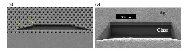
**Figure 3.17:** SEM images of cross-cuts created by the ion beam in: (a) Au film showing the cylindrical shapes of the milled holes as indicated by the yellow arrows, (b) a 300 nm Ag film evaporated on a glass substrate in order to measure the actual thickness of the film by imaging.
