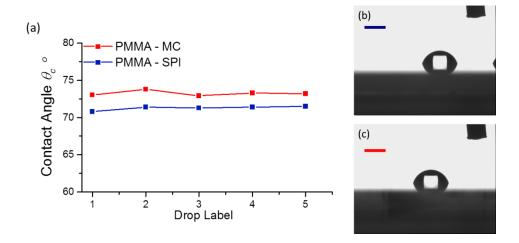
**Figure 3.23:** (a) The value of contact angle measured for a set of 5 different drops on the surface of (b) PMMA mixed with SPI before and (c) after irradiation with UV.
