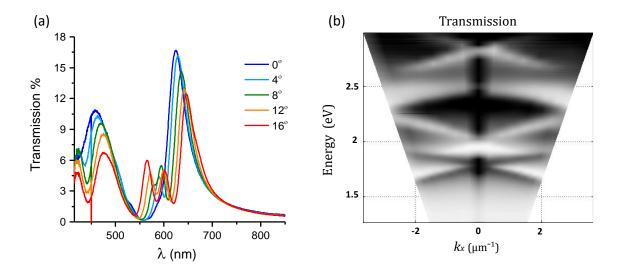
**Figure 3.9:** (a) The zero-order transmission spectra as a function of incident angle of the light in TM mode. Spectra were taken every  $4^{\circ}$  up to  $16^{\circ}$  for hexagonal array in Ag ( $a_0 = 400 \text{ nm}$ , hole diameter = 205 nm, film thickness = 200 nm). (b) The energy-momentum dispersion of the same spectra present in (a) in addition to their symmetric values for negative angles. The bright lines represent peaks and dark ones represent dips.
