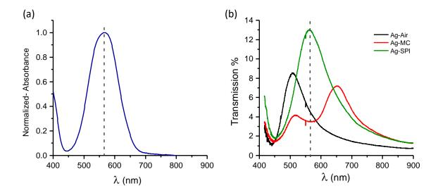
**Figure 3.13:** (a) Normalized absorbance of MC with a maximum centered at 565 nm (dashed line). (b) Transmission spectra at normal incidence for the same hole-array ( $a_0 = 250$  nm, D = 120 nm) at different interfaces. The red curve represents the splitting of peaks due to the coupling of MC transition band (centered at the vertical dashed line) with the plasmonic resonances.
