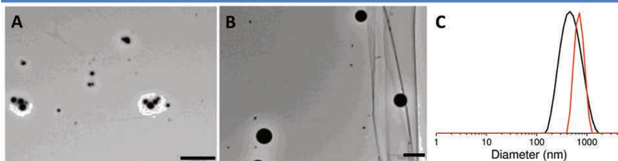
Figure 43 | A-B. TEM images of TATT in a chloroform/toluene/methanol mixture (50/45/5 vol%) A. before irradiation ( c = 1 mM, scale bar: 1 \mu\text{m} ) and B. after irradiation ( c = 0.1 mM, scale bar: 1 \mu\text{m} ); C. Distributions of hydrodynamic diameters observed for TATT before (black) and after (red) light irradiation for 90 minutes.
