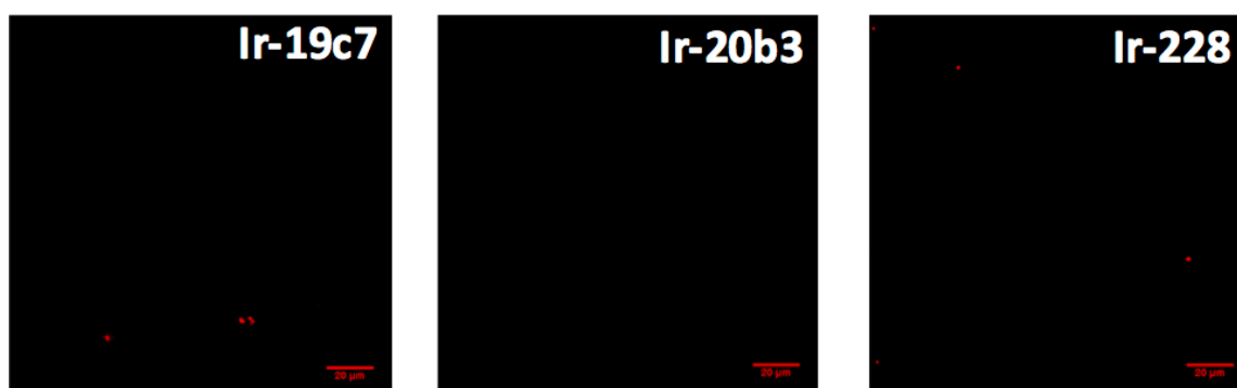
Figure 6.10. Confocal Images of the control experiments (monolayer, capture antibody and detection antibody when cTnI complex is absent). Scale bar 20 μm. Luminescence images were recorded live on a Zeiss LSM510 Meta confocal microscope using a 40× oil immersion objective lens (NA 1.4) and a 488 nm argon ion laser applied for Iridium labelled antibody imaging.
