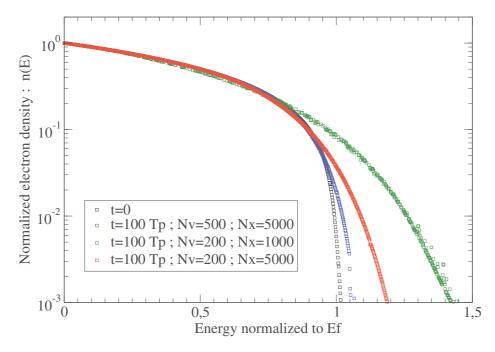
FIGURE 4.13: Energy densities of the electrons for the equilibrium distribution function of nickel films with  $L=100L_{\rm F}$  and  $\sigma=1L_{\rm F}$  ( $L_{\rm F}\simeq 0.1~nm$ ). The equilibrium case correspond to the black squares. The other cases correspond to the energy densities after 100~Tp (without exciting the system) with different phase space grids.
