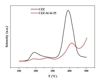
Figure 4- 9 CO<sub>2</sub>-TPD profiles for CZZ and CZZ-Si/Al-25
