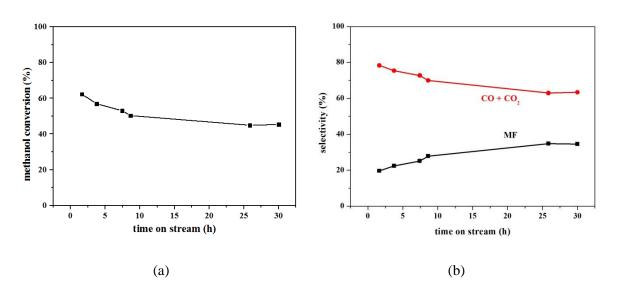
Figure 4- 15 Methanol conversion (a) and products selectivity (b) for CZZ catalyst
