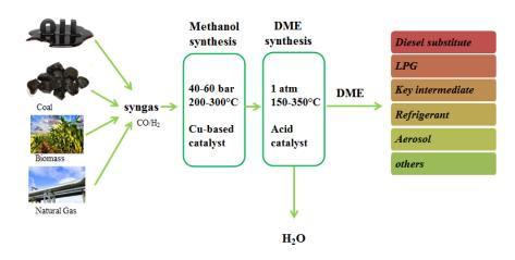
Figure 1-4 Schematic diagram for traditional DME synthesis
