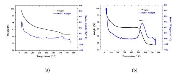
Figure 4- 6 TGA profiles of CZZ and of CZZ-Si/Al-25
