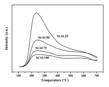
Figure 3- 5 NH<sub>3</sub> desorption profiles for Al-TUD-1
