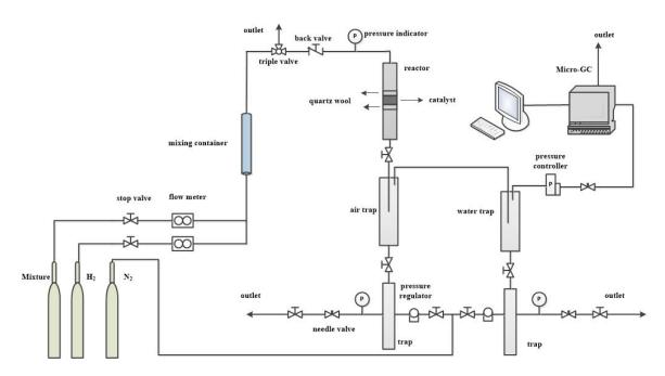
Figure 2-4 Scheme of setup for direct DME synthesis from CO<sub>2</sub>/H<sub>2</sub>
