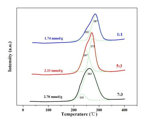
Figure 4- 21 TPR patterns for bifunctional catalysts
