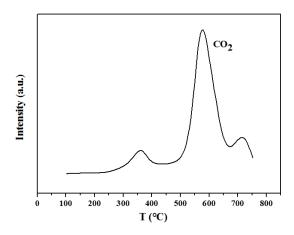
Figure 4- 7 CO<sub>2</sub> profile from CZZ-Si/Al-25 TGA analysis
