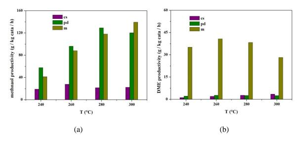
Figure 5- 10 Methanol (a) and DME (b) productivity
