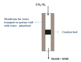
Figure 6- 1 Schematic diagram of a membrane reactor
