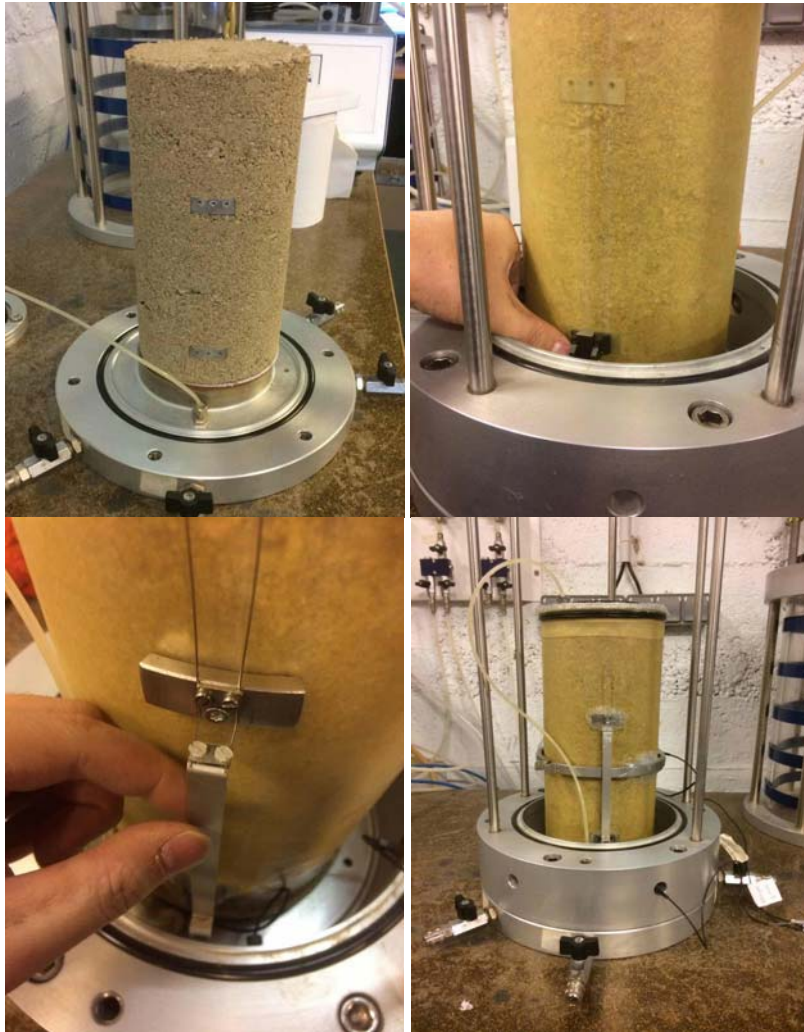
Figure A.4. Photos of the fixing devices for the displacement transducers on the UGM sample
