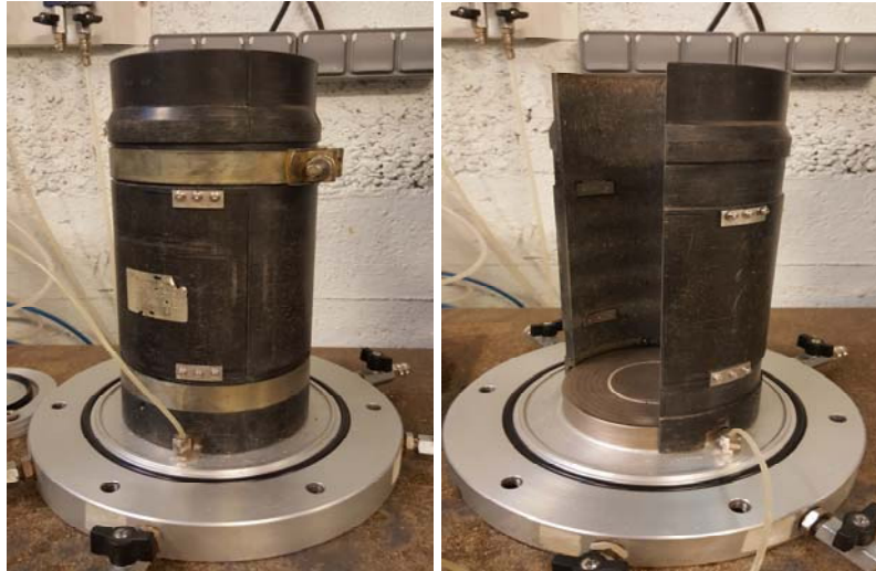
Figure A.3. Photos of the fixing devices for the displacement transducers on the compaction mould
