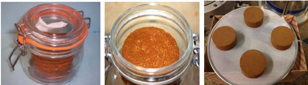
Figure II.10. Jar containing the sample of Missillac sand and gauze-plate for drying
