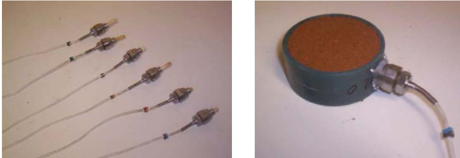
Figure II.14. Porous probes and the sample connected with a measuring probe
