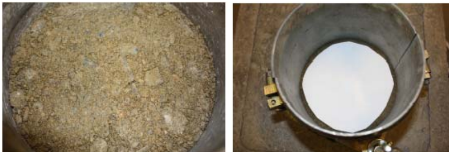
Figure II.11. Filter paper inserted in a sample of UGM Maraîchères
