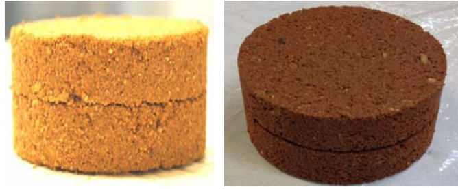
Figure II.9. Missillac sand samples of suction measurement with filter paper method (M4.0 and M15.3)
