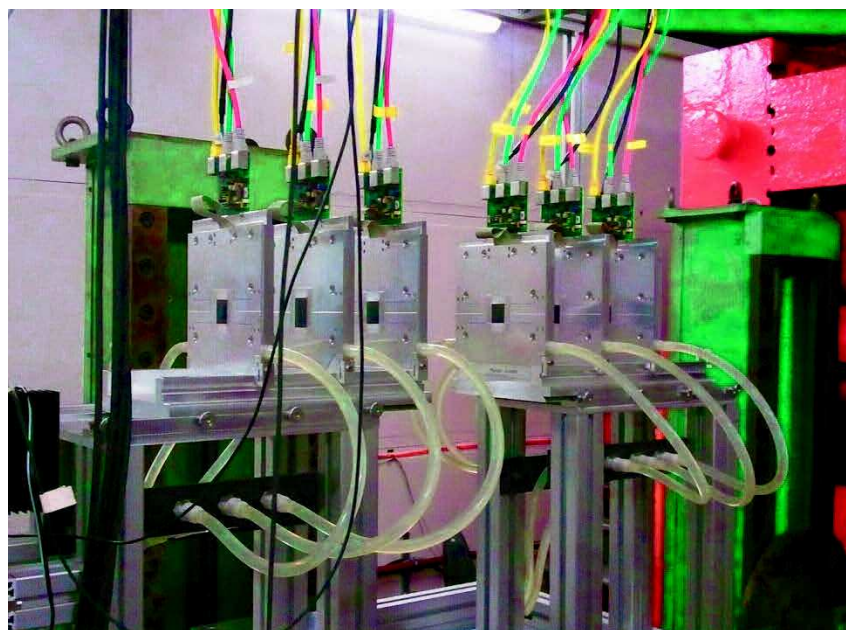
Figure 2.8: Photo of EUDET telescope using Mimosa26 sensors
