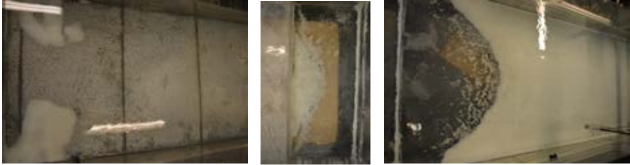
Figure 4.59 Sediment distribution at 3 L/s 3 hours after particle release
