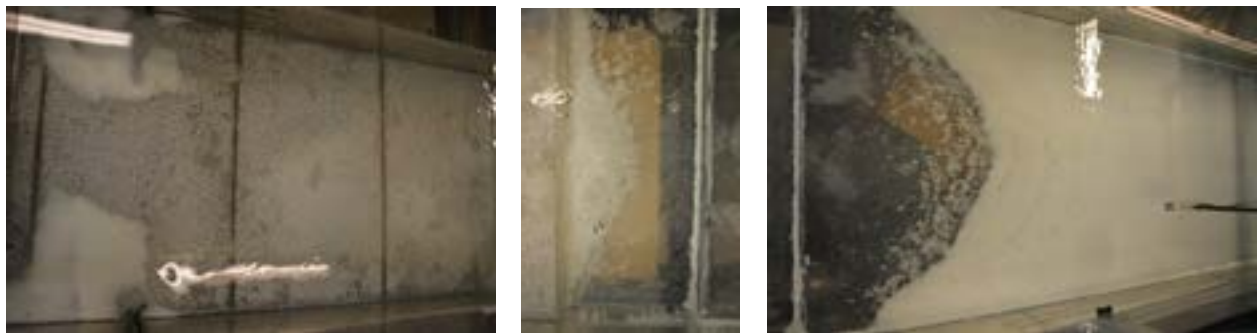
Figure 4.58 Sediment distribution at 3 L/s 2 hours after particle release
