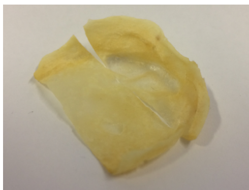
Figure 76 – Image of DOUBLE DYNAMIC recycled after neutralisation and evaporation of DOUBLE DYNAMIC from a THF solution
