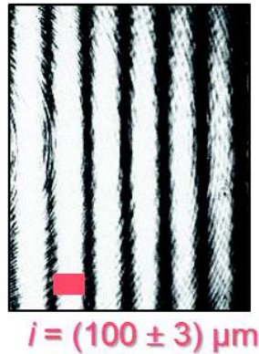
Figure 5.2: The measurement of the fringe spacing through the projection of the fringe pattern on a CCD camera. 1 fringe is equal to 100 \pm 3 \mu\text{m} .
