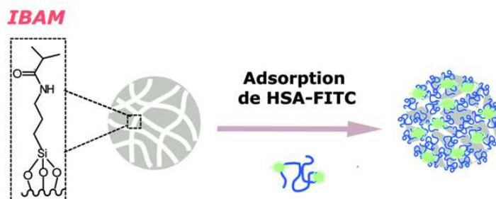
Figure 4-13: Strategy of the formation of a HSA-FITC coating on mesoporous silica particles
