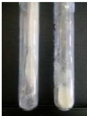
Figure 4.4. Binary mixture ratio 1:1 of ketoprofen with HPMC (left) and ketoprofen with PVP (right) after 6 months were stored under accelerated stability test conditions
