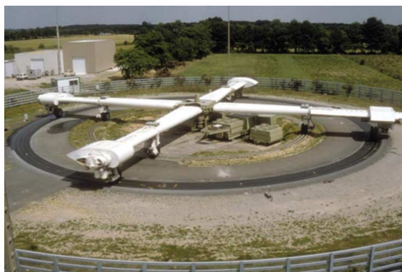
Figure II.1.3: Pavement fatigue carousel at IFSSTAR in Nantes, France [NGU 13]
