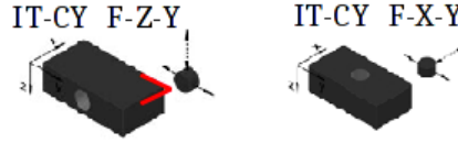
Figure III.3.13: Extraction of specimens from slabs in the study of Hofko et al. [HOF 16]
