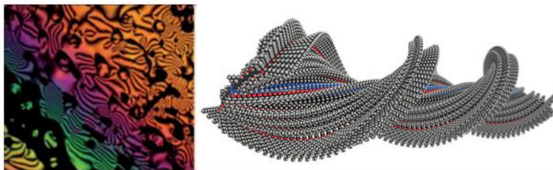
Figure 1.4: Examples for self-assembly utilized in science. Left: Nematic phase of liquid crystalline molecules. 88 © 2010 Wiley; Right: Ordered supramolecular polymer, that forms a twisted nanoribbon. 89 © 2012 Science
