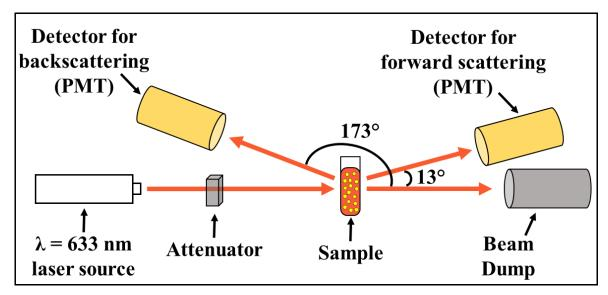
Figure 3.4: Scheme of a DLS size analyzer.
