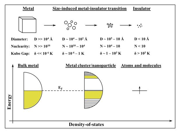
Figure 2.2: Schematic diagram showing the size-depend evolution of the energy level of metals. (Adapted from Ref.<sup>3</sup>).
