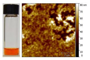
Figure 6.3: Optical and AFM pictures of PDI-4T in  $THF/H_2O$  (kept in dark).
