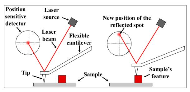
Figure 3.6: Schematic representation of the AFM setup.
