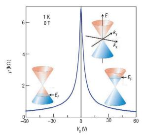
Figure 2. 17: Ambipolar electric field-effect in single-layer graphene on 300 nm SiO2 dielectric layer. The insets show its conical low-energy spectrum E(k), indicating changes in the position of the Fermi energy EF with changing gate voltage  $V_g$ . Positive (negative)  $V_g$  induce electrons (holes). Reproduced with permission from Ref. 149
