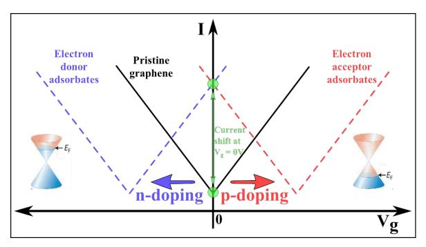
Figure 2.18: Schematic of the current shift given by the presence of adsorbates on graphene and rGO surface.
