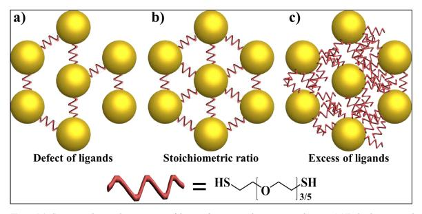
**Figure 5.1**: Cartoon explaining the importance of the use of proper stoichiometric ratio between AuNPs binding sites and free thiol groups in solution. a) Effect of a defect of the ligands in solution. b) Effect of proper stoichiometric ratio. c) Effect of excess of ligands in solution.
