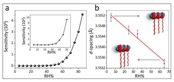
Figure 2.12: Effect of water absorption on CS-DMV nanofibers. (a) Electrical sensitivity response of the chemiresistive humidity sensors. (b) Change in the  $\pi$ - $\pi$  stacking distances between the building blocks as a consequence of water absorption (probed by performing XRD measurements at different RH). Adapted with permission from Ref. <sup>107</sup>
