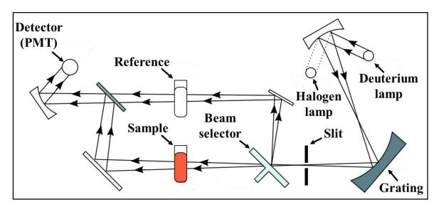
Figure 3.3: Scheme of a double beam UV-Vis spectrophotometer.
