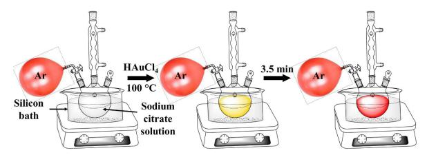
Figure 3.1: Schematic of the synthesis for the water-soluble gold nanoparticles.
