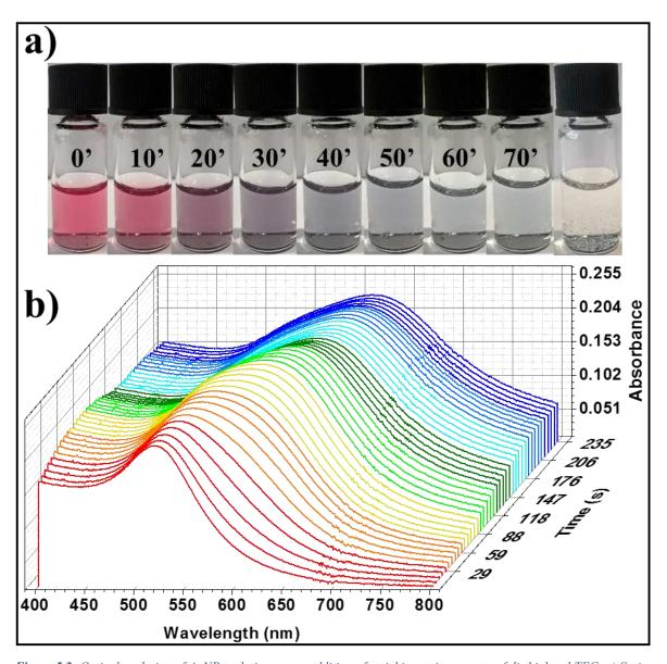
**Figure 5.2**: Optical evolution of AuNPs solutions upon addition of stoichiometric amounts of di-thiolated TEG. a) Series of optical photographs of the solution recorded with steps of 10 minutes and after one day (last picture). b) Evolution of the UV-Vis absorbance spectra within the first 4 minutes upon addition of the ligand solution.
