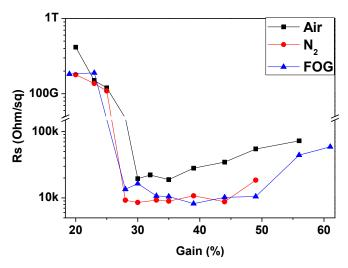
**Figure 7.9:** Sheet resistance for 2.8 nm thick GO film as a function of laser intensity (%) for three different atmospheres (FOG = 5% H<sub>2</sub>, 95% N<sub>2</sub>).
