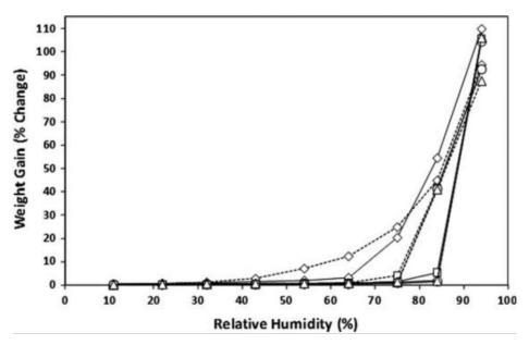
Figure 4.10: Vapor sorption isotherms of various MW PEGs measured by automated gravimetric moisture analysis at each relative humidity. ( $\Diamond$ ) PEG 1450, ( $\Box$ ) PEG 3350, (O) PEG 6000, ( $\Delta$ ) PEG 8000. Solid lines (-) and dashed lines (-) are isotherms measured at 25° C and 40° C respectively. Reprinted with permission from Ref. <sup>19</sup>
