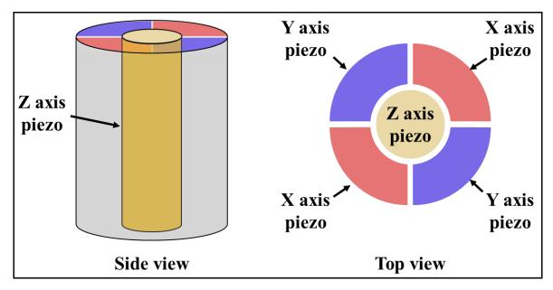
Figure 3.7: Schematic of a XYZ piezoelectric scanner tube.
