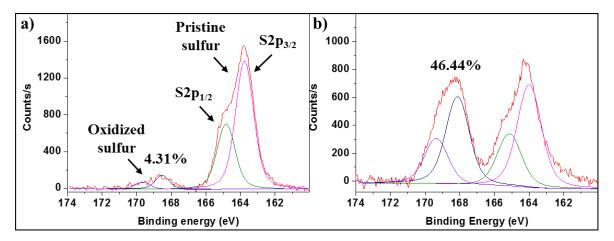
Figure 6.7: XPS spectra of PDI-4T drop cast solutions. a) Solution kept in dark for 6 months. b) Solution exposed to white light for 20 hours (power density =  $100 \text{ mW/cm}^2$ ).
