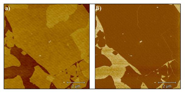
Figure 7.1: AFM a) height (Z scale = 11 nm) and b) phase images of GO from Graphenea on SiO<sub>2</sub>.
