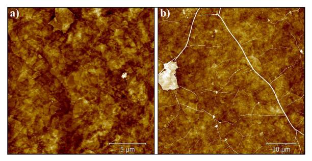
Figure 7.2: AFM topographical image of GO uniform films with different thickness. a) 3 nm thick film (image Z scale = 14 nm). b) 17 nm thick film (image Z scale = 60 nm).
