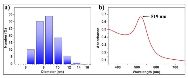
Figure 3.2: Characterization of the water-soluble AuNPs. a) Dynamic light scattering. b) UV-Vis absorbance spectra.
