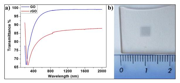
**Figure 7.13**: Optical properties of rGO. a) Comparison between the optical transmittance spectra of GO (unexposed area) and rGO (exposed area). b) Photograph of sample with 4x4mm² wide window of rGO drawn on a uniform 17 nm thick GO film on quartz substrate.
