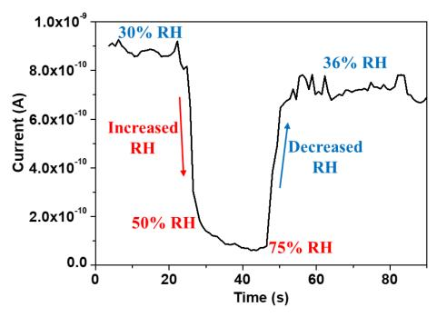
Figure 4.5: Effect of environmental humidity on the electrical characteristics of single domains of 2D AuNPs networks (constant bias applied =  $1\ V$ )
