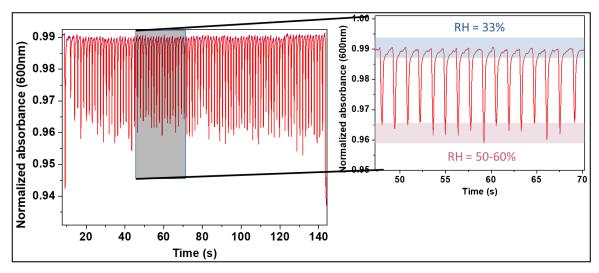
Figure 4.9: Optical response of AuNPs networks exposed to short pulses of humid air (pulses frequency = 2 Hz). Inset showing a zoom-is of the highlighted region of the plot.
