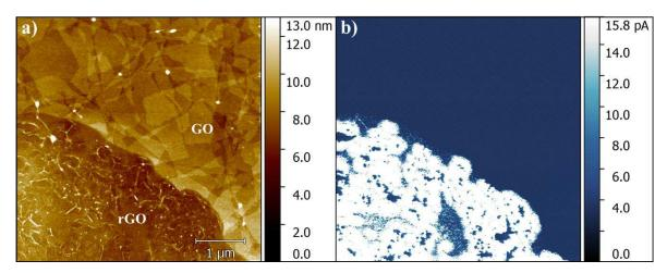
Figure 7.12: C-AFM characterization at the border between exposed and unexposed areas on 2.8 nm thick GO. a) Topography image. b) Electrical current map.
