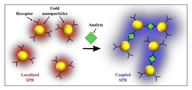
Figure 2.8: Schematic representing the working principle of colorimetric chemical sensors based on AuNPs LSPR.
