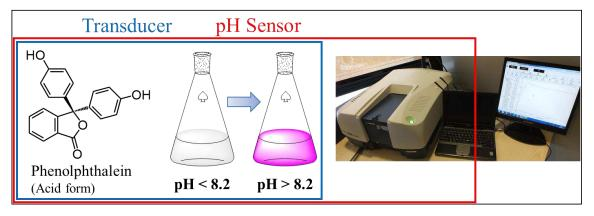
Figure 1.1: Example of a complex pH sensor made phenolphthalein transducer and a UV-Vis spectrophotometer as optical sensor.
