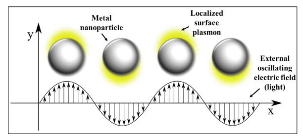
Figure 2.6: Schematic of the localized surface plasmons formation.
