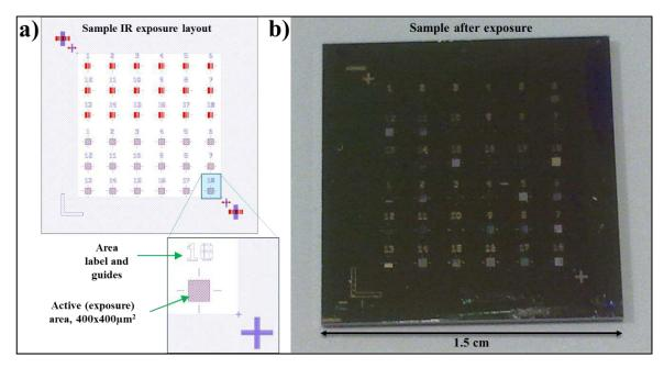
Figure 7.4: Layout for the systematic study of GO Laser reduction. a) Scheme of the layout. b) Optical picture of a sample series on SiO<sub>2</sub> after exposure.
