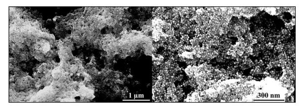
Figure 5.3: SEM images of AuNPs/TEG porous 3D networks.
