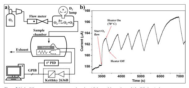
Figure 7.16: L-rGO ozone sensors test setup and results. a) Scheme of the used setup b) L-rGO electrical current response to absorption and desorption of ozone vs time under various cycles.
