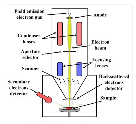
Figure 3.9: Structure of a scanning electron microscope.
