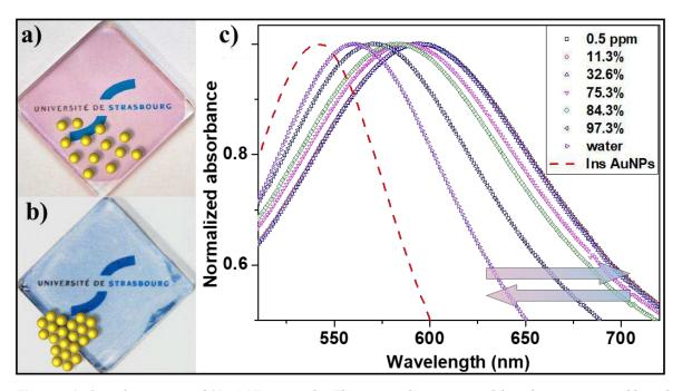
Figure 4.6: Optical properties of 2D AuNPs networks. The increased environmental humidity causes a visible and reversible change of color from blue (b) towards red (a). This change of color is given by a gradual shift and sharpening of the UV-Vis extinction band which moves gradually from 595 to 560 nm, towards a state of completely insulated AuNPs (c).
