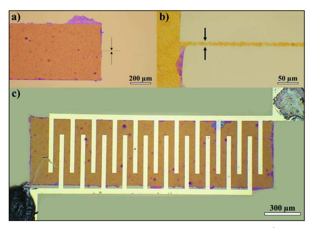
Figure 7.15: Optical micrograph of large area L-rGO structure for ozone sensing devices. a)  $600 \times 2000 \ \mu m^2$  L-rGO after unused GO removal shows the presence of GO residuals attached to the edges of the structure. b) Zoom-in showing a 10  $\mu$ m wide rGO line. c) Ozone sensor structure with interdigitated electrodes.
