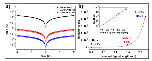
Figure 5.6: Electrical behavior and average resistance of AuNPs-based electrical devices (channel length =  $2.5 \mu m$ ). a) Average I-V curve of bare AuNPs (used as reference), AuNPs networks with TEG and HEG ligands. b) Plot of average device resistance versus the nominal length of the fully extended ligands.
