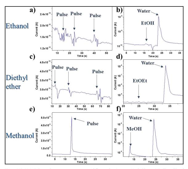
Figure 6.10: PDI-4T electrical response upon exposure to different solvent's vapors (Applied bias = 5 V; Channel length =  $5 \mu m$ ). a) Pulses of ethanol. b) Comparison between ethanol and water. c) Pulses of diethyl ether. d) Comparison between diethyl ether and water. e) Pulses of methanol. f) Comparison between methanol and water.
