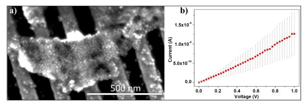
Figure 4.4: Electrical characterization of AuNPs 2D networks. a) SEM image of a single domain bridging the gold electrodes. b) I-V characteristics recorded in a two-terminal device configuration.
