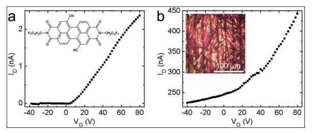
Figure 2.10: Electrical characteristics of rylene-based transistors. Transfer characteristics for (a) a spun-cast thin film transistor (molecular structure shown in inset), and (b) a fibers transistor based on the same molecule (optical micrograph of the supramolecular fibers on interdigitated source-drain electrodes shown in inset). Channel length =  $10 \mu m$ , Vd = 10 V. Reprinted with permission from Ref. 99
