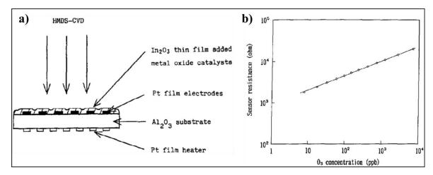
Figure 1.4: In<sub>2</sub>O<sub>3</sub> resistive ozone sensor reported by Takada et al in 1993. a) Design of the device. b) resistance response at different ozone concentrations. (Images reprinted with permission from Ref.<sup>23</sup>)
