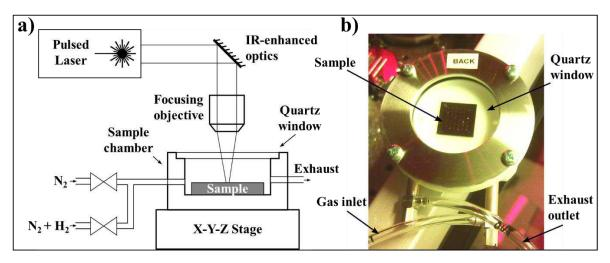
Figure 7.3: Laser writer setup used for the Laser assisted reduction of GO. a) Scheme of the setup. b) Optical picture of a sample inside the sample chamber.
