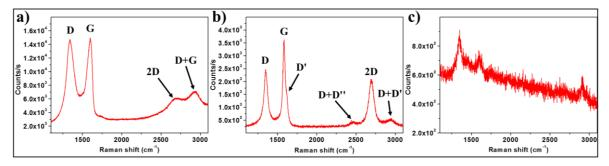
Figure 7.7: Raman spectra of GO. a) Pristine GO. b) Optimally reduced. c) Damaged by too high power density.
