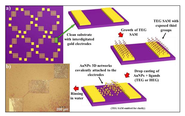
Figure 5.4: Optimized procedure for the fabrication on 3D AuNPs/OEG based electrical devices. a) Flowchart of the process. b) Optical micrograph of the resulting device.
