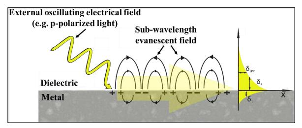
Figure 2.5: Schematic of the formation and propagation of SPs at the metal/dielectric interface.
