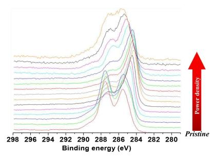
Figure 7.5: XPS C1s spectra of GO films exposed to IR laser at different power densities.
