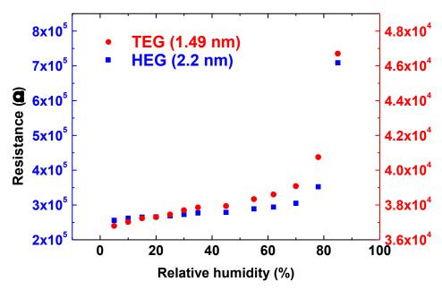
Figure 5.9: Calibration curves of AuNPs TEG and HEG-based humidity sensors.
