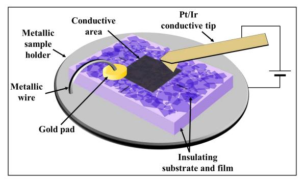
Figure 3.8: Experimental configuration employed for the C-AFM characterization of L-rGO in chapter 7.
