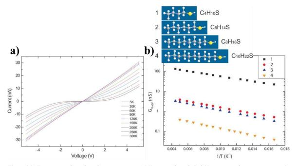
**Figure 2.3**: Temperature dependent charge transport. a) I-V curves of interlinked 2D nanoparticles arrays measured at variable temperatures from 5K to 300K. b) Zero-voltage conductance of the nanoparticle arrays as a function of inverse temperature for nanoparticle arrays with different inter-particle distances. Adapted from Ref. 15 with permission of the Royal Society of Chemistry.
