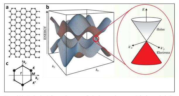
**Figure 2.16**: (a) Graphene's honeycomb structure. (b) Band energy dispersions calculated via tight binding approximations (inset highlights the conical-shape dispersion around the Dirac point). (c) First Brillouin zone. Adapted from Ref. <sup>151</sup>
