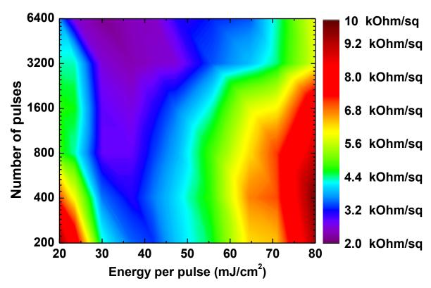
Figure 7.10: Effect of amount of pulses and energy per pulse on the sheet resistance of  $17 \pm 1$  nm thick L-rGO under  $N_2$  atmosphere.
