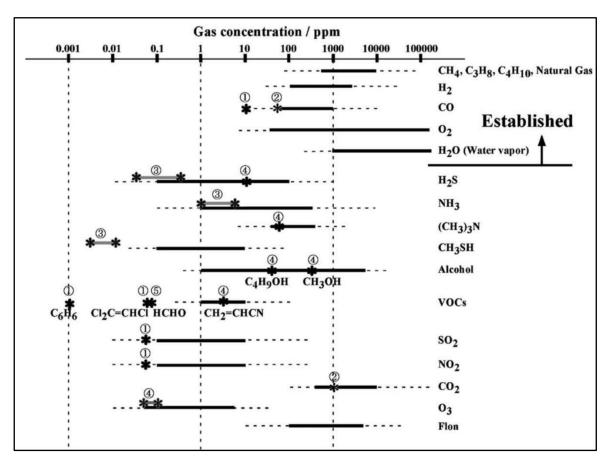
Figure 1.2: Concentration levels of typical gas components concerned. Star marks indicate the standards of the gases legislated in Japan by (1) Environmental Standard, (2) Ordinance on Health Standards in the Office, (3) Offensive Odor Control Law, (4) Working Environment Measurement Law, and (5) Ordinance by Ministry of Health, Labour and Welfare. (Image reprinted with permission from Ref.<sup>2</sup>).
