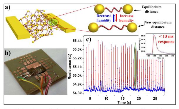
Figure 5.8: Electrical resistive humidity sensors based on AuNPs/OEG 3D porous networks. a) Schematic of the sensing process. b) Picture of the device setup used for the sensor's characterization. c) Measurements of response speed, reversibility and stability of the final devices (constant bias applied = 500 mV).
