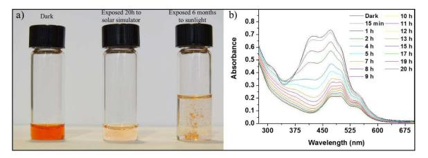
*Figure 6.4:* Evolution of PDI-4T solution's optical properties upon light exposure with white light (power density: 100 mW cm<sup>-2</sup>). a) Optical pictures. b) UV-Vis absorbance spectra.
