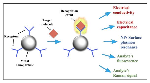
**Figure 2.1**: Schematic summarizing the metal nanoparticles-based sensing methods (Red = electrical readout. Blue = Optical readout monitoring the NPs features. Green = Optical readout monitoring the analytes features).
