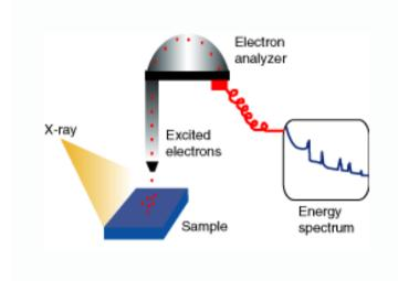
Figure 5.3 Schematic representation of the principle of XPS. Figure taken from reference 3.
