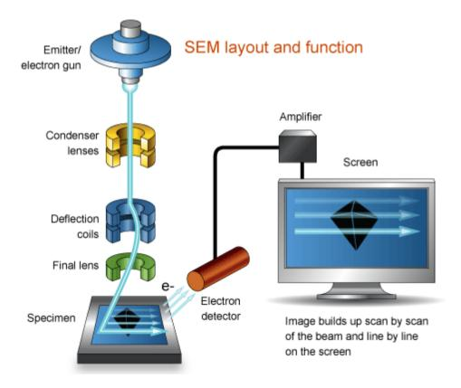
Figure 5.5 Schematic representation of a SEM and its principle. Figure taken from reference 4.
