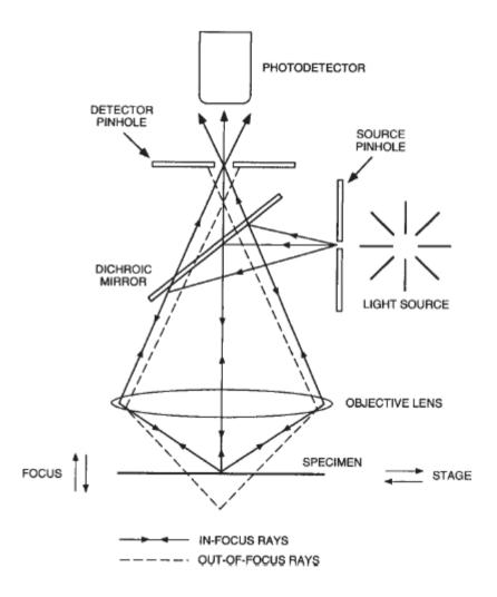
Figure 5.7 Principle of CLSM. Figure taken from reference 2.
