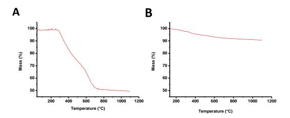
Figure 2.18 TGA of (A) S-Cy5-BMONPs and (B) S-Cy5-MSNPs.
