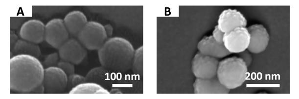
Figure 2.16 SEM pictures of (A) S-Cy5-BMONPs and (B) S-Cy5-MSNPs.
