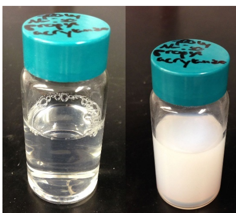
Figure 1.4 Behavior of a thermo-responsive polymer below the LCST (left) and above the LCST (right). Source: wikimedia
